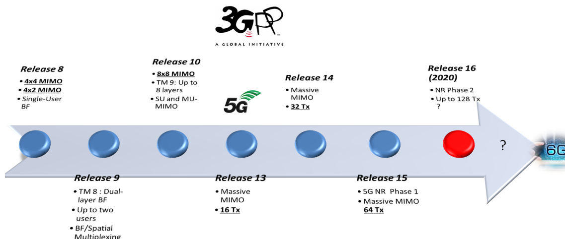
Figure 1.3: 3GPP Releases-From MIMO to massive MIMO. This figure displays the evolution from Release 8 to the up-coming Release 16.
