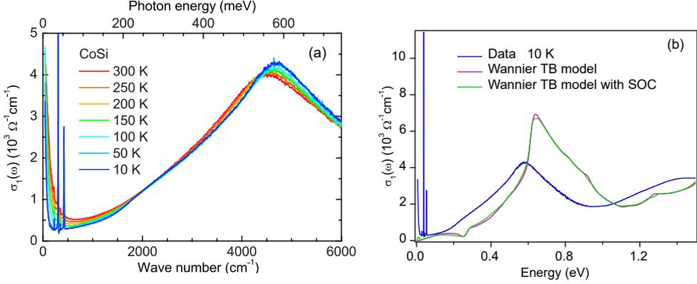
**Figure 4.3:** Experimental optical conductivity of CoSi. (a) Temperature-dependent optical conductivity spectra  $\sigma_1(\omega)$  of a CVT-grown CoSi (001) crystal. (b) Measured optical conductivity at 10 K along with the Wannier tight-binding calculation with and without spin-orbit coupling at 10 K. Adapted from Ref. [114].
