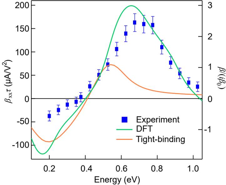
**Figure 5.1:** Experimental CPGE spectrum of RhSi (blue squares) compared to the DFT calculation for  $\mu = -30$  meV and temperature  $T = 300$  K (solid green line), and the tight-binding model (Eqs. 2.34–2.35) presented in Sec. 3.4.2 (solid orange line) for the parameters  $v_1 = 1.95$ ,  $v_p = 0.77$ , and  $v_2 = 0.4$ . Both theoretical calculations are computed with a constant broadening  $\eta = 100$  meV. Reproduced from Ref. [75].
