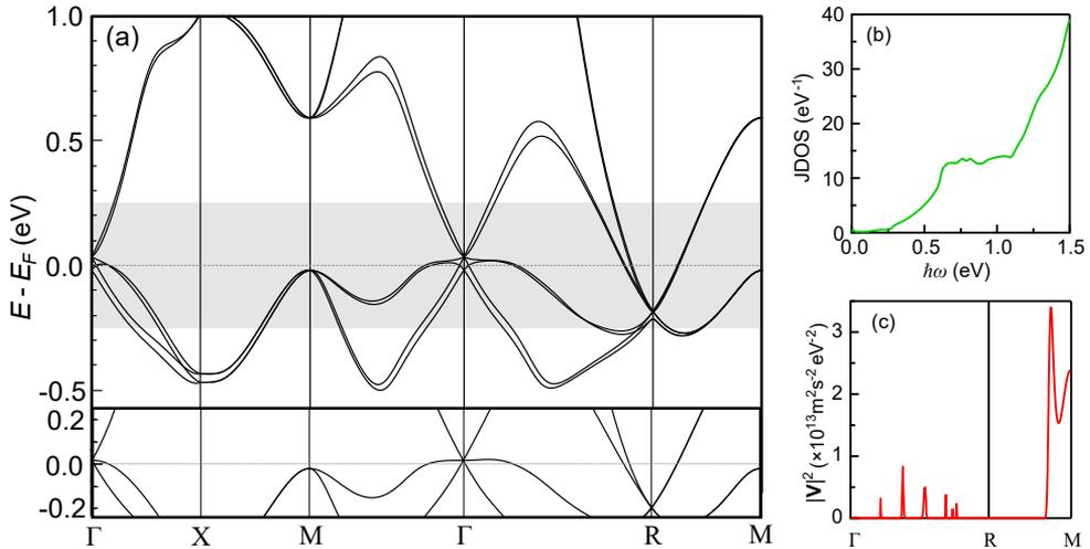
**Figure 4.2:** DFT band structure, JDOS, and matrix elements of CoSi. (a) Band structure of CoSi with spin-orbit coupling. The bottom inset shows the band structure without spin-orbit coupling in the same shaded energy window of (a). (b) Joint density of states as a function of energy. (c) Momentum-resolved matrix elements that contribute to the 0.62 eV interband transition along  $\Gamma - R - M$  direction. Adapted from Ref. [74].
