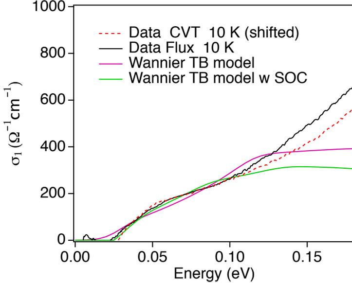
**Figure 4.6:** Interband optical conductivity in CoSi from measurements in both CVT- and flux-grown samples (red and black curves) along with Wannier tight-binding calculations without (pink curve) and with (green curve) spin-orbit coupling. Reproduced from Ref. [114].
