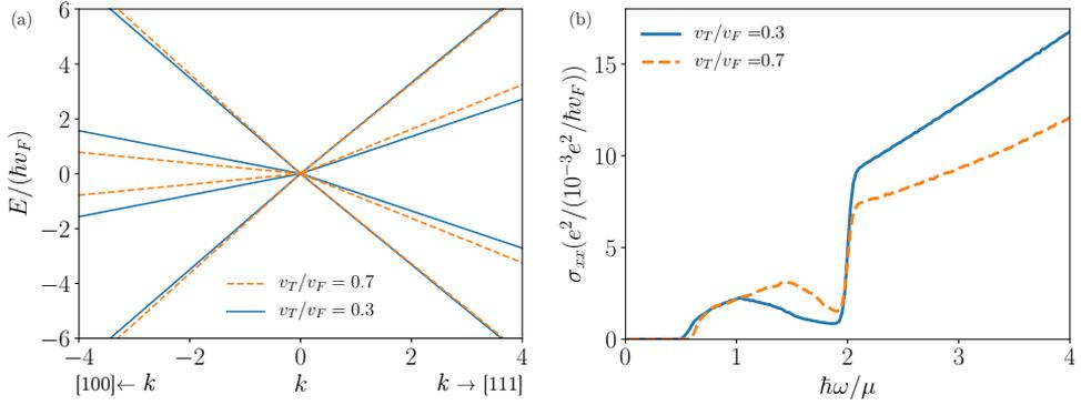
**Figure A.1:** Optical conductivity of a tetrahedral fourfold fermion. (a) Band structure and (b) optical conductivity corresponding to the tetrahedral fourfold fermion with two different values of the ratio  $v_T/v_F$  (see Eq. 2.27).
