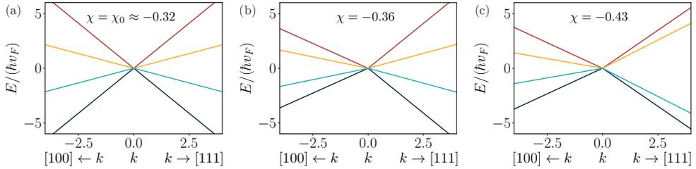
**Figure 2.3:** Band dispersion for symmetric and non-symmetric fourfold fermions. (a) For  $\chi = \chi_0 = \arctan(-1/3)$ , the fourfold Hamiltonian in Eq. 2.23 has full rotational symmetry. We refer to this case as symmetric fourfold fermion. (b) For  $\chi \neq \chi_0$  the Hamiltonian loses full-rotational symmetry, leading to an asymmetry in the band structure, which becomes more asymmetric (c) as  $|\chi - \chi_0|$  grows.
