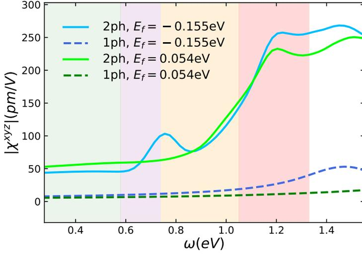
**Figure 5.6:** Calculated different components of SHG from two-photon (solid sky blue line) and one-photon (dashed royal blue line) transitions with Fermi energy  $E_f = -0.155$  eV, as well as two-photon (solid green line) and one-photon (dashed dark green line) transitions with Fermi energy  $E_f = 0.054$  eV and scissors potential  $\Delta = 1.23$  eV. The total SHG susceptibility is plotted in Fig. 5.4 (c). Reproduced from Ref. [76].
