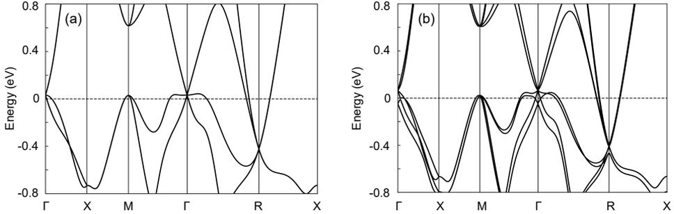
**Figure 4.8:** DFT band structure of RhSi (a) without spin orbit coupling, and (b) with spin orbit coupling. It hosts a threefold fermion at  $\Gamma$  and a double-Weyl fermion at  $R$  without spin orbit coupling. They split into a spin-3/2 fourfold node and a Weyl node at  $\Gamma$ , and a sixfold double spin-1 node and a twofold Kramers node at  $R$ , when spin orbit coupling is included. Reproduced from Ref. [75].
