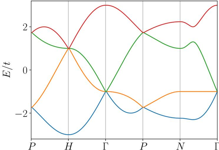
**Figure 2.4:** Band structure of the tight-binding model for SG199 in Eqs. 2.29–2.30. This model features a threefold crossing at the  $\Gamma$  point with energy  $\mu_{\Gamma}/t = -1$  and at the  $H = (-\pi, \pi, \pi)$  point at energy  $\mu_H/t = 1$ . Additionally, it hosts two Weyl nodes at the  $P = (\pi/2, \pi/2, \pi/2)$  point with energies  $\mu_{W_1}/t = -1.732$  and  $\mu_{W_2}/t = 1.732$ , and two Weyl crossings with opposite charge at  $-P$ .
