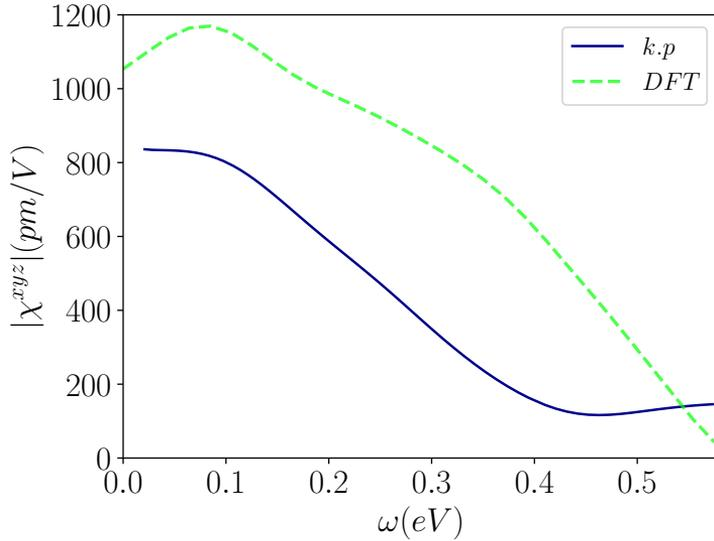
**Figure 5.8:** Comparison between the second-harmonic response obtained for the  $k \cdot p$  model (blue line) at  $E_f = -0.27$  eV and DFT calculations (dashed green line) at  $E_f = -0.14$  eV. Both curves are calculated with  $\Delta = 0$  eV and  $\eta = 0.1$  eV. Reproduced from Ref. [76].
