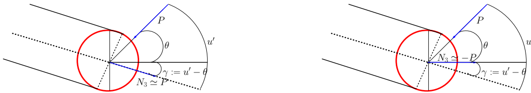
Figure 2.6 – Left, the assumption for the normal force in the Engesser beam–column model. The normal force is parallel to the beam axis. Right, the assumption for the normal and shear forces in the Haringx beam–column model. The normal force is parallel to the normal of the deformed cross-section.
