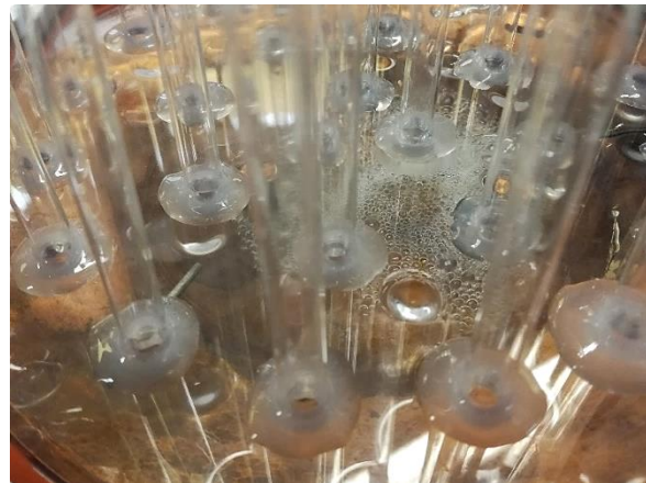
a) pentane, Ø5 mm, \dot{Q}_{tot}/\dot{Q}_{cp} = 75/55 W, charge 5
