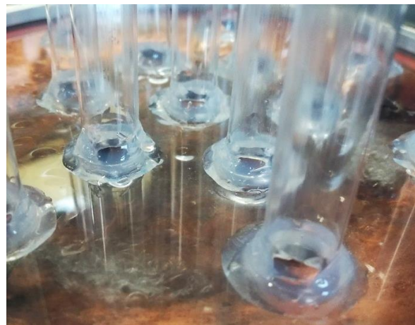
b) HFE-7100, \varnothing 11 mm, \dot{Q}_{tot}/\dot{Q}_{cp} = 120/77 W, charge 16
