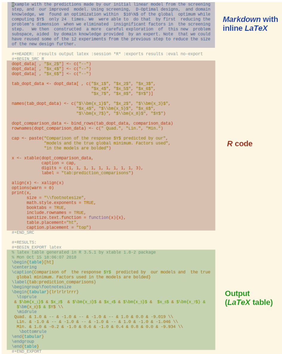
Figure 8.2: Excerpt of the org file generating our CCGRID paper [48, 37], showing code, generated output, and markdown text
