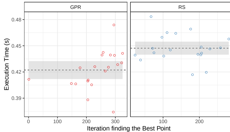
Figure 12.9: Best bicg configurations and iterations that found them, for Gaussian Process Regression with Expected Improvement acquisition function (GPR), and uniform Random Sampling (RS), with a budget of 400 measurements.
