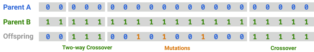
Figure 3.6: Some ways of producing offspring from two parents with binary chromosomes. Crossover splits parent chromosomes and combine the resulting pieces. In general, pieces from multiple splits can be combined. Mutations are introduced randomly and correspond to flipping bits on binary chromosomes.
