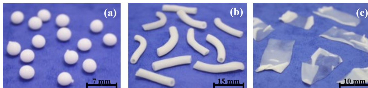
Figure V-3: Photographs of the QQ (a) beads (b) hollow cylinders and (c) sheets.
