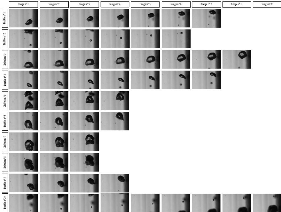
Figure II-12 : Series of images recorded at the top of the membrane (Window I) for the determination of the properties of bubbles generated in the ALMBR under an air flowrate of 0.90 \text{ Nm}^3 \cdot \text{h}^{-1} \cdot \text{m}^{-2} with a riser width of 15 mm (the time between two consecutive images of a series is 5 ms).
