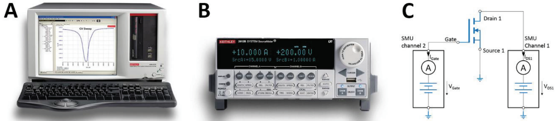
Figure 54: Source measure units to characterize semiconductors with high accuracy and high resolution down to the fA range. Both channels of the source measure units are required to measure one field effect transistor.
