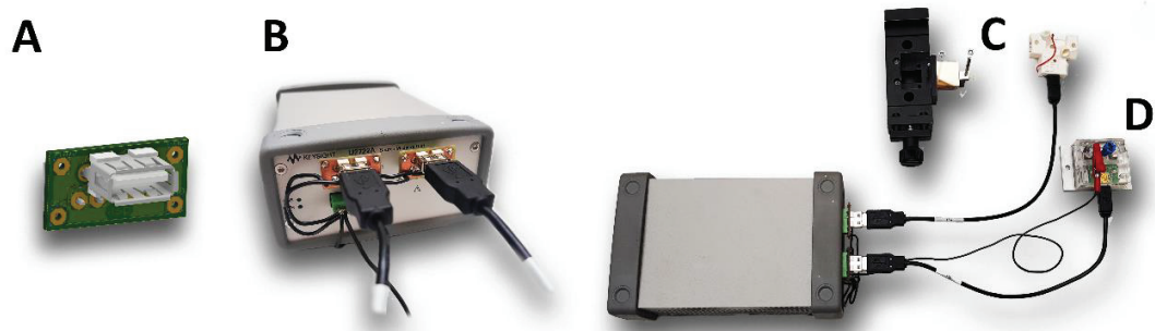
Figure 62: A: Connector board to a standard USB-A plug for both drain-source channels. B: Connected USB cables to the SMU. The gate electrode is connected to the shield of the USB cable for the gFET/SPR flow cell and to a wire for the Micrux flow cell, shown in C. D: The connection of the Keysight U2722A source meter unit to the Micrux flow cell with a USB cable and a wire for the liquid gate electrode. The gFET/SPR flow cell and Micrux gFET flow cell are connected for parallel measurements.
