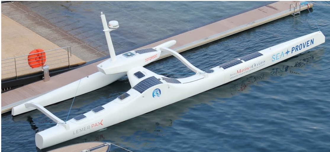
Figure 5.1: The ASV Sphyrna, 17m long. It is a proa (South Pacific design), consisting of two unequal length parallel hulls. It is extremely stable, even at high wind force.
