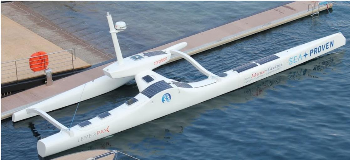
Figure 5.1: The ASV Sphyrna, 17m long. It is a proa (South Pacific design), consisting of two unequal length parallel hulls. It is extremely stable, even at high wind force.
