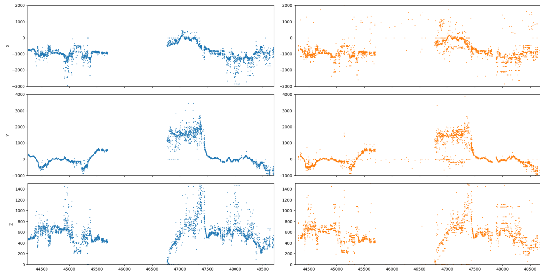
Figure 5.9: Raw coordinates of the Sperm Whale during the last two dives, in the keel antenna reference space. The blue points are from the DBSCAN filtering. The orange points are from the baseline [137].
