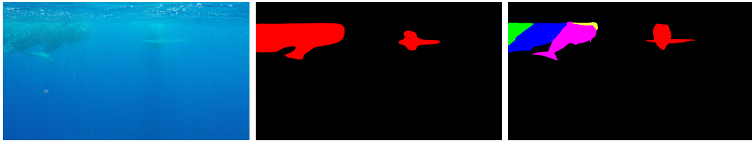
Figure 6.10: Image (left) with its semantic segmentation (middle) and its instance segmentation (right)
