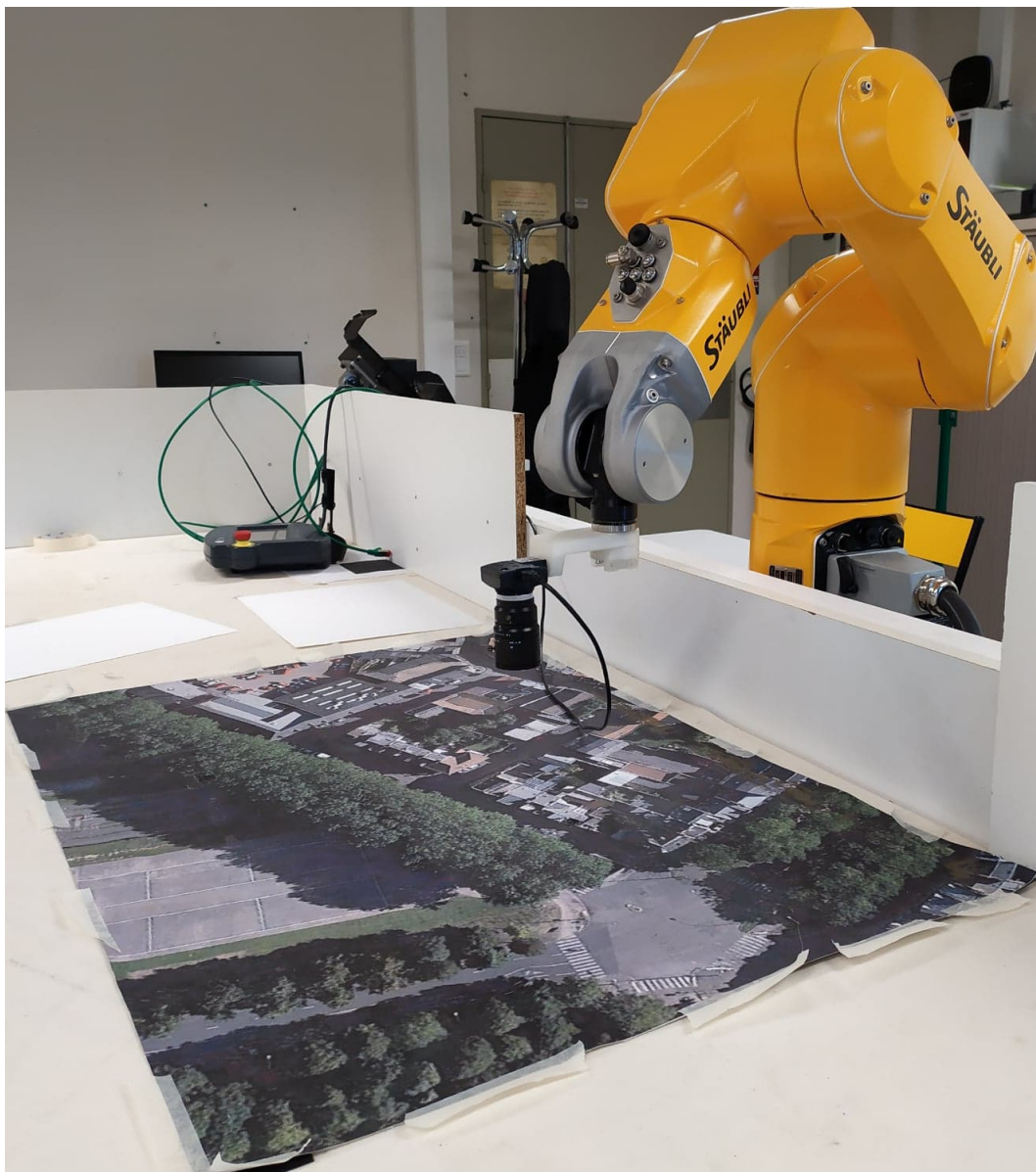
Figure 6.1: Experimental setup. The uEye camera is mounted on the end-effector of the robot. The latter travels through the planar textured scene.
