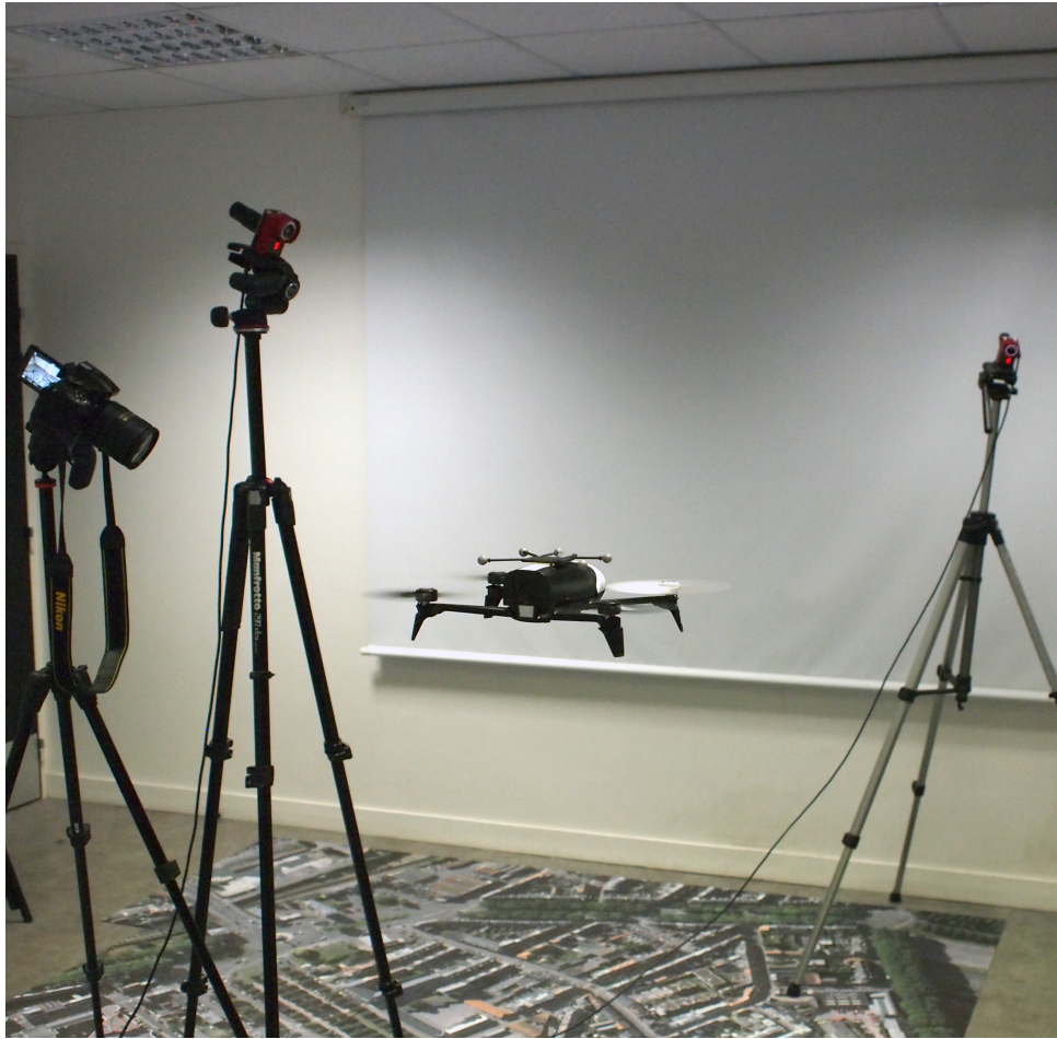
Figure 3.5: Setup for indoor experimentation. The Bebop 2 flies over the scene with the onboard camera virtually pointing downwards. The Optitrack system tracks records the pose of the rigid frame of markers attached to the robot. Additionally, a Nikon D5200 records video of the experiment.
