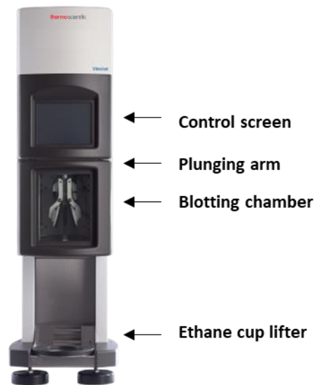
Figure 1.12 : Schematic of a plunge-freezing robot. Example of a Vitrobot Mark IV and its main components. The gridboxes are placed in the ethane cup, which will be lifted towards the blotting chamber. The grid is placed in the plunging arm and after applying the sample, the blotting arms (white) will blot the grid and it will be plunged into the ethane. Reproduced from ( https://www.thermofisher.com/ch/en/home/electron-microscopy/products/sample-preparation-equipment-em/vitrobot-system.html ).
