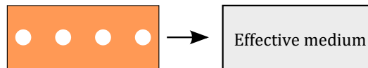
Figure 1.3 – Homogenisation approach, in which a composite material is represented by an effective medium.
