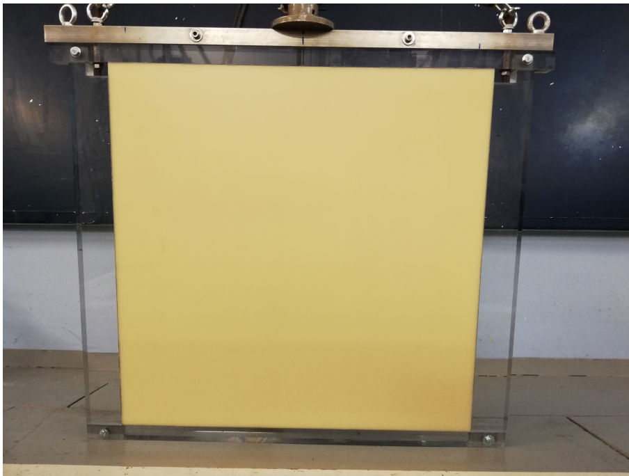
Figure 4.13 – Polyurethane panel comprising 6% of micro-balloons. The panel is held by a Plexiglas frame.
