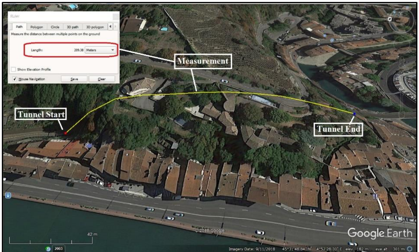
Figure 4.19. Tunnel length measurement using Google Earth
