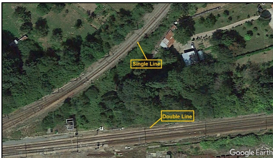
Figure 4.3. Single and Double Line Originating from A Railway Station
