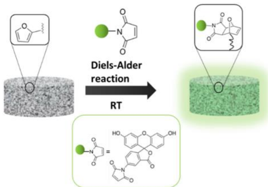
Figure 4.16 : Schematic illustration of furfuryl-containing CG-40 before and after loading with N -(5-fluoresceinyl)maleimide via DA cycloaddition.
