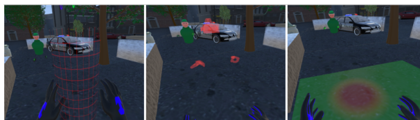
(b) Different representations of the collaborator's position in the shared physical workspace: a virtual cylinder (left), a ghost (middle) and a safe-navigation space on the floor [68].
