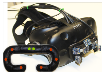
(c) Vibro-tactile actuators integrated in HMD cushions [107].
