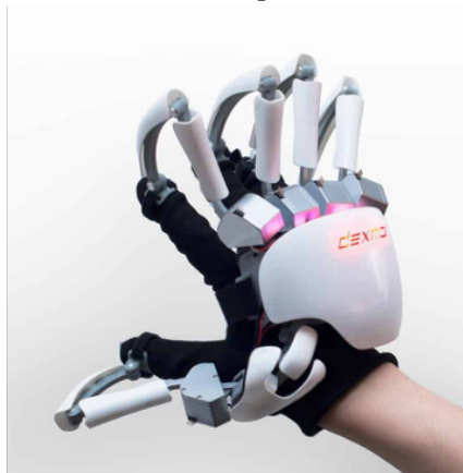
(c) Dexmo ® , a wearable mechanical exoskeleton. © Dexta Robotics
