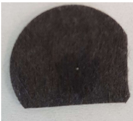
Figure IV.23: FeNi 3 @Ni sample used for the ILSEM study. The little hole in the centre and the two cut edges of different sizes allowed to identify different positions in the carbon felt.
