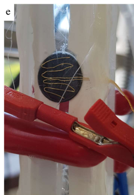
Figure II.8: (a) PMMA cell (b) Counter-Electrode with the sewn gold wire electrical contact (c), (d), (e) the carbon felt working electrode with the single, fork and rake shape gold wire current collector, respectively.
