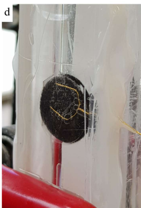
Figure II.8: (a) PMMA cell (b) Counter-Electrode with the sewn gold wire electrical contact (c), (d), (e) the carbon felt working electrode with the single, fork and rake shape gold wire current collector, respectively.
