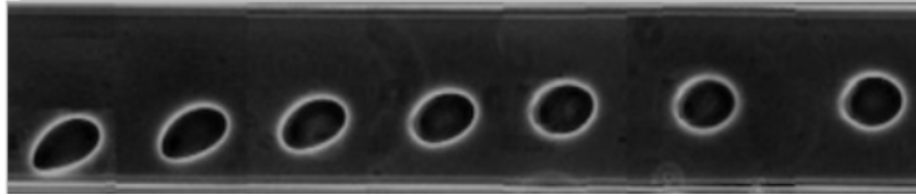
Figure 1.8: Soft microparticles (vesicle) in the vicinity of interfaces experienced hydrodynamic interactions that push them away from the wall. Image from Ref. [78]
