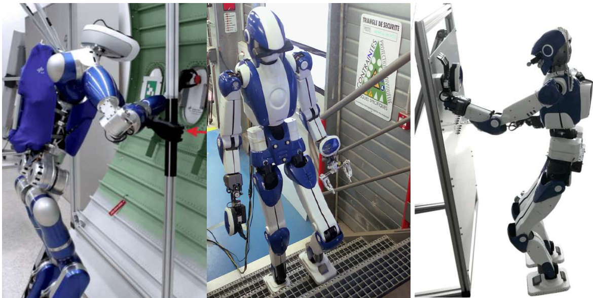
FIGURE 1.10 – TORO and HRP-4 humanoid robots operating multi-contact Kheddar et al. (2019) and stair climbing Caron et al. (2019) tasks in the industrial environments.
