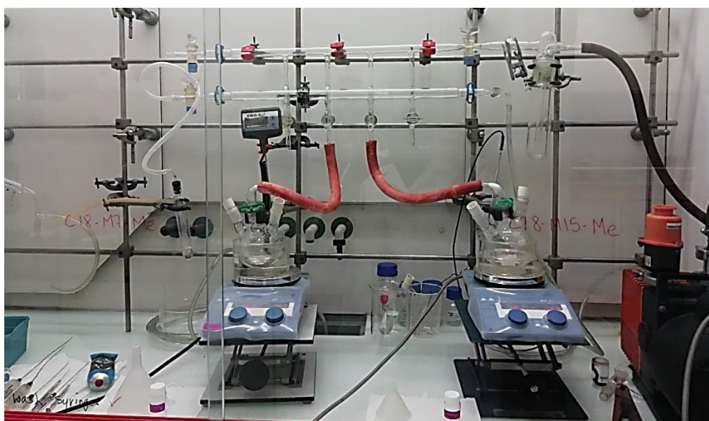
Figure 1: Apparatus for reaction under inert atmosphere.
