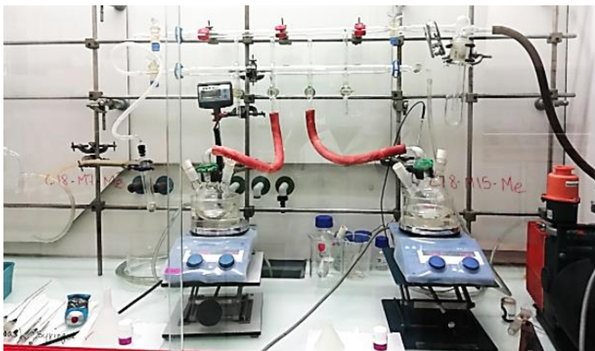
Figure 2.2: Apparatus for the post-grafting reaction under an inert atmosphere.
