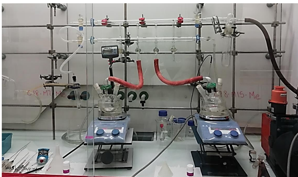
Figure 1: Apparatus for reaction under inert atmosphere.
