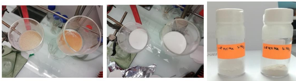
Figure 9: Materials before (left) and after (middle) drying. At the right, samples as they have been storage. The obtained powders do not disperse in water, only in ethanol.
