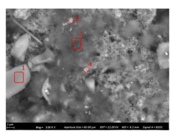
Figure 4.29. SEM images of Ni/LSCF<sub>prop</sub>/RSiC 8/5 catalyst post steam reforming of toluene at 550 °C
