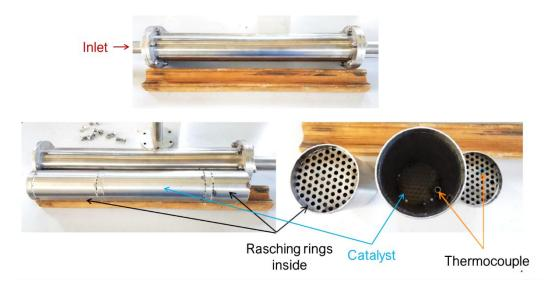
Figure 5.2. Catalytic reactor used at pilot plant scale
