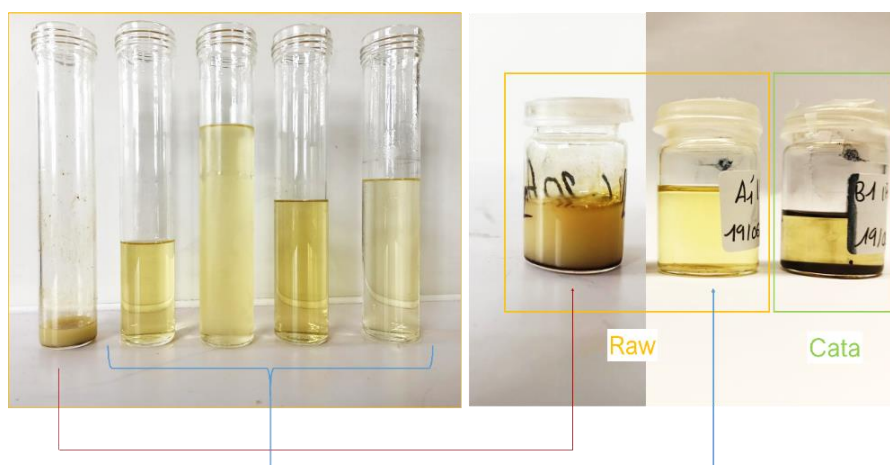
Figure 5.23. First tar sampling recorded through raw line and cata line during catalytic test with residues
