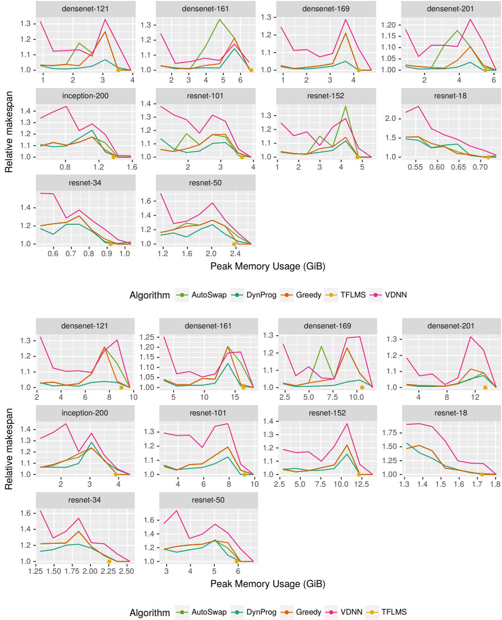
Рис. 3.5: Relative makespan (with respect to the lower bound) obtained by different algorithms for different memory limits. Experimental results are provided for image size 224 and batch size 32 (top), image size 500 and batch size 16 (bottom).
