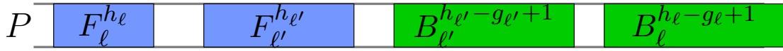
(a) Worst case. Memory needed to store the activations: g_\ell a_{\ell-1} + g_{\ell'} a_{\ell'-1} (reached between F_{\ell'} and B_\ell ).
