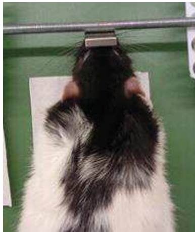
Figure 9. Experimental set-up for the assessment of magnetic field effect on IVT injected MNPs. Since the MNPs were already in the back of the eye we changed the position of the magnet in order to assess the effect of the magnetic field on the movement of the particles
