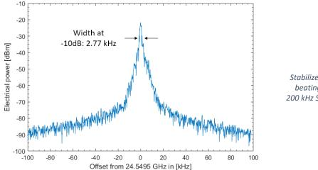
Figure 3-28 Stabilized laser fundamental beating RF spectrum with 200 kHz Span and 300 Hz RBW and VBW
