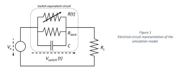
$V_{switch}$  voltage is used to estimate the electrical DC field accelerating the photogenerated carriers. Using Kirchhoff's circuit law, we can write equation (5).
