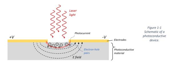
When the illumination is turned off, the current flow will disappear as the carrier generation stops and all the free charges are recombining with the holes. The time of recombination is called the carrier lifetime.
