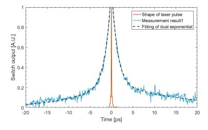
Figure 2-37 Fitting of the exponentials on both sides of an example result curve; orange curve is the femtosecond laser pulse after fibre propagation
