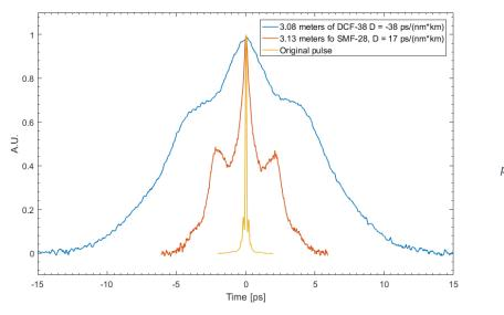
Figure 20 pulse shapes after propagating in different dispersive fibres
