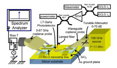
Figure 1-22 Illustration of the mixing setup with photoswitch and two heterodyned single mode lasers as the LO source Source: E. Peytavit et al. Applied Physics Letters, 2013, [35]
