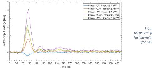
Figure 2-27 Measured pulses with the fast sampling oscilloscope for SA2-2 switch
