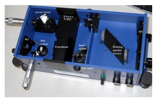
Figure 3-10 Top view of the Femtochrome FR-105XL autocorrelator
