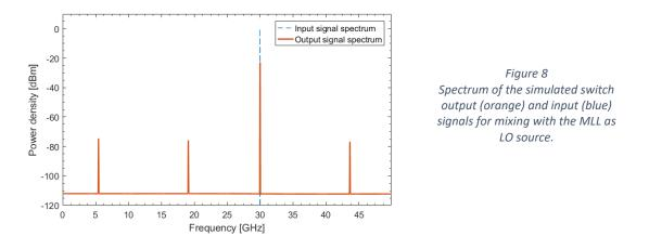
We can observe the mixing products at  $f_{RF} - m^* f_{LO}$ , and the feedthrough signal too at 30 GHz.
