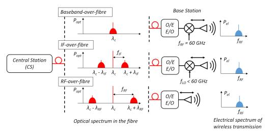
Figure 4-35 Illustration of the 3 RoF scenario. O/E: Optical to electrical converter; E/O: electrical to optical converter
