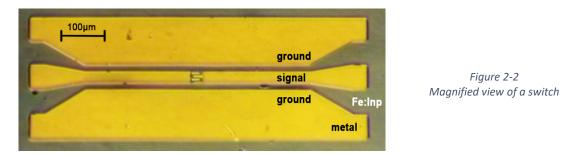
The CPW line has a characteristic impedance of 50  $\Omega$ . Close to the sample edges the CPW widens, while keeping the 50  $\Omega$  impedance. This widened CPW makes it possible to connect the switch to coplanar electrical RF probes during the experiments. The geometry allows to use probes with pitch sizes of 100  $\mu$ m or 150  $\mu$ m. All the switch samples on both substrates are identical in size and material, the only differences are the geometry of the interdigitated structures.
