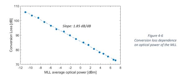
It is difficult to predict the saturation value where the conversion loss would be the lowest, it is depending on semiconductor material properties and physical effects like the saturation of the
