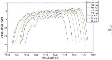
Figure 3-9 Optical spectrum envelops versus bias current at 21°C temperature
