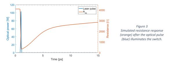
In the simulation the contributions of the holes and electrons are weighted thanks to the different mobilities (see below), as it was observed from our experiment in II/3.4.e. The resistance drop also results in a voltage drop on the switch, as seen in Figure 4 with blue curve, the orange curve shows the voltage at the circuit output on  $R_L$ .
