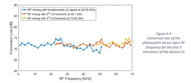
The results show that the conversion loss has a variation of 7 dB around 72 dB over the full 69 GHz wide RF frequency range. The performance is uniform for all three local oscillator harmonics, which shows that at least the first 3 beating signal of the MLL produces the similar RF power.
