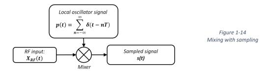
According to the Shannon criteria (equation (22)), the sampling frequency should be at least twice as the maximum frequency of the input RF signal in order to be able to reconstruct all the information.
