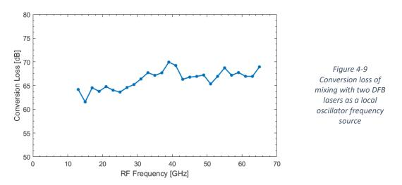
The measurement shows a conversion loss around 67 dB, which is slightly increasing with higher RF frequencies. The value is 5 dB better than in the case of the MLL laser (see Figure 4-4), which is also caused by the higher optical power used here. However, a complete comparison of the conversion loss could be misleading, because in the MLL case the RF signal is generated by the
