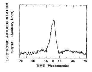
Figure 2-29 LT-GaAs photoconductor response as measured by F.W. Smith et al., Appl. Phys. Lett., Vol 54, 1989 [15]
