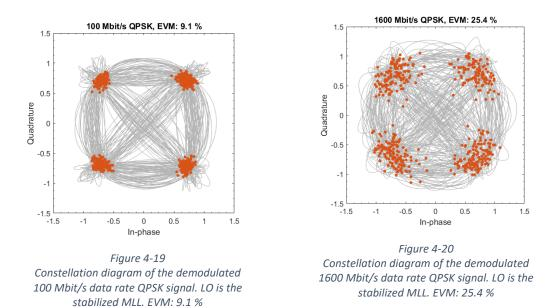
The calculated values of BER with the stabilized MLL as LO are below the value of 10<sup>-3</sup> for data rates up to 1600 Mbit/s, in the literature this value is considered as a practical limit of error rate for
