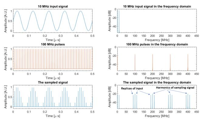
Figure 1-15 Illustration of a sinusoidal signal sampling in the time domain and the frequency domain
