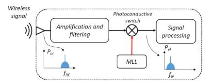
Figure 4-34 Photoswitch based optoelectronic mixers used as a downconverter of high carrier frequency signals
