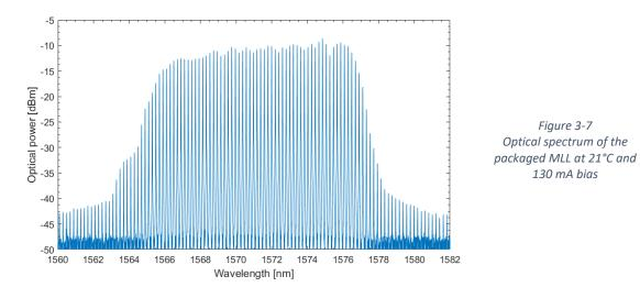
The laser is emitting in the 1570 nm wavelength range and contains 40 optical modes in an 8 nm wide 3 dB bandwidth, therefore most of the spectrum lies in the optical L-band (1565-1630 nm).
