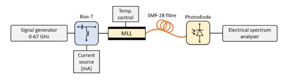
Figure 3-20 Setup for the external RF modulation of the MLL
