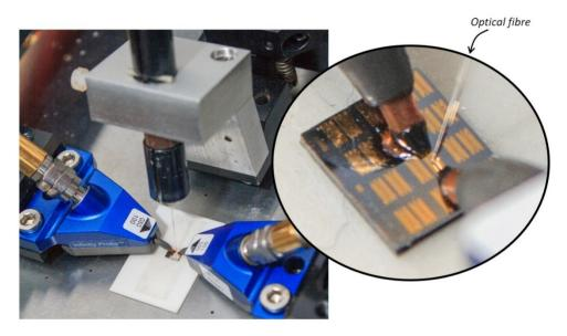
Figure 4-1 Photoswitch sample in the RF probe station with two RF probes and fibre probe. Inset: magnified view of the connected switch
