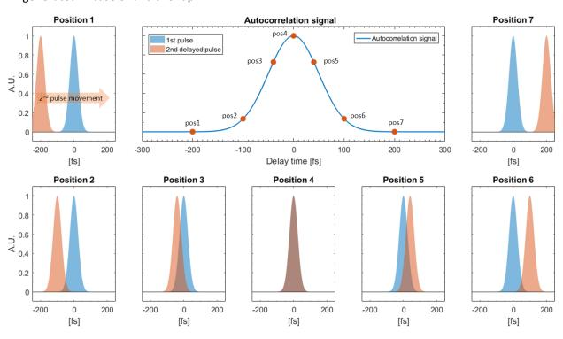
the autocorrelation curve. The dark orange area is the overlap of the two curves, the third beam is generated in case of this overlap.
