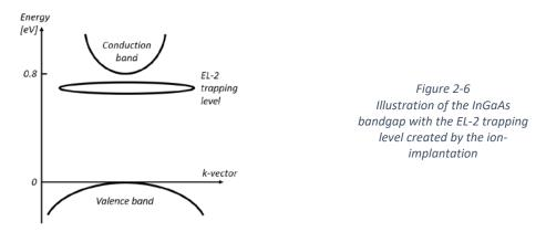
The InGaAs bandgap of 0.8 eV means that it is sensitive to 1.5  $\mu$ m wavelengths. These wavelengths are widely used in today's telecommunication networks, making the photoconductive switch compatible with modern systems.
