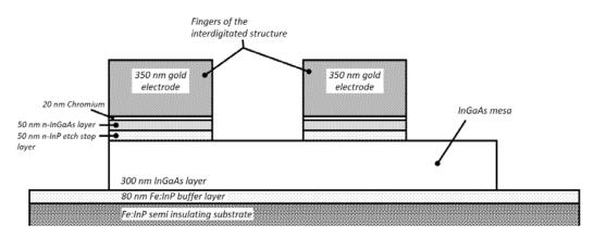
Figure 2-5 Cross-section of the photoconductive switch. Vertical and horizontal dimension are not in scale
