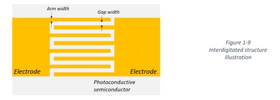
The neighbouring arms are connected to opposite electrodes, creating an interweaving structure. The fingers are increasing the area where the carriers can be collected but on the other hand the illuminated area is decreasing by the shadowing effect of the metal electrodes.
