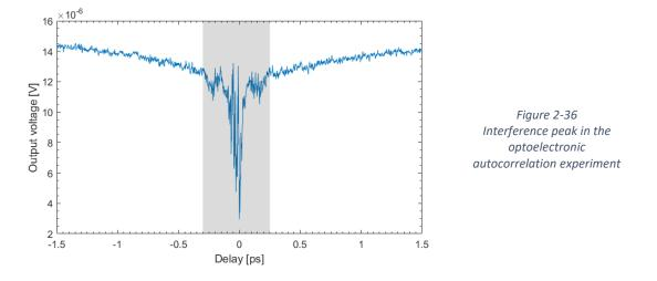
Therefore, while calculating the exponential fitting, this interference will not play a role in the fitting values. Because of this, we do not have information about the real peak value, it can be just assumed form the crossing point of the two side fittings on the curve, however it is not important for the measurement to know this peak value. The identified time range for the interference is marked with grey in Figure 2-36 (the illustration shows the maximum interference), it is 0.55 ps wide.
