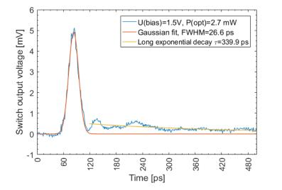
Figure 2-28 Fitting example of the fast sampling oscilloscope result measuring SA2-2
