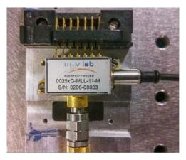
Figure 3-2 MLL laser in a butterfly package
