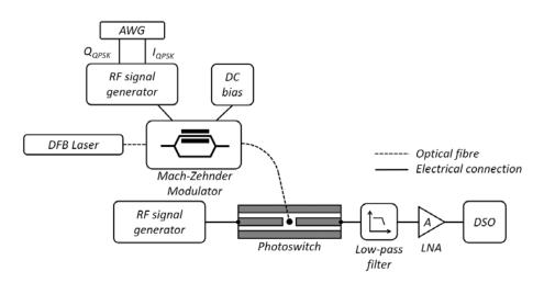
Figure 4-26 Setup for the data-stream downconversion. Electrical signal as the local oscillator source, data-stream is intensity modulated on a DFB laser's signal
