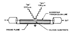
Figure 1-2 Photoconductive switch design by Auston. Source: D. H. Auston, Appl. Phy. Lett. Vol. 26, No 3, 1975 [2]
