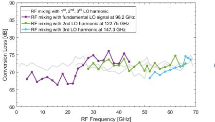
Figure 4-5 Conversion loss of the photoswitch versus input RF frequency for the 4<sup>th</sup>, 5<sup>th</sup> and 6<sup>th</sup> harmonics of the optical LO
