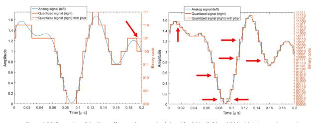
Figure 1-26 Illustration of the jitter effect on the quantized signal for 3 bits (left) and 5 bits (right), sampling rate is 200 MHz.
