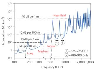
shows the free-space loss and resonance peaks up to 3 THz [9]. Suggested bands chosen for longand medium distance, and indoor applications are marked in the figure.
