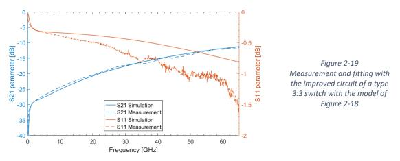
We can see that the simulation has a very good fit on the measured S<sub>21</sub> values. Despite the accurate model, the role of the circuit elements is not properly understood, it needs further investigation to understand the physical meanings behind all the elements of the circuit.
