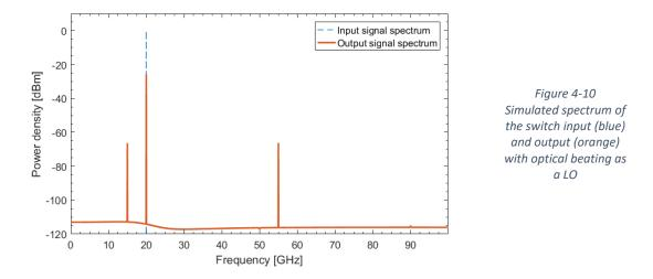
The higher peak of the orange curve is the feedthrough signal from the input. The two lower peaks are the IF signals at 15 GHz ( $f_{LO} - f_{RF}$ ) and at 55 GHz ( $f_{LO} + f_{RF}$ ). Both of it has a power level of -66.3 dBm, which corresponds to 66.3 dB of conversion loss. This value is in the same range as our measurement, illustrated in Figure 4-9. See APPENDIX A for a detailed description.
