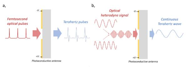
Figure 1-7 **a**: Terahertz pulse generation and **b**: CW terahertz generation with photoconductive antenna
