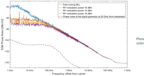
Figure 3-21 Phase noise of MLL with external RF modulation
