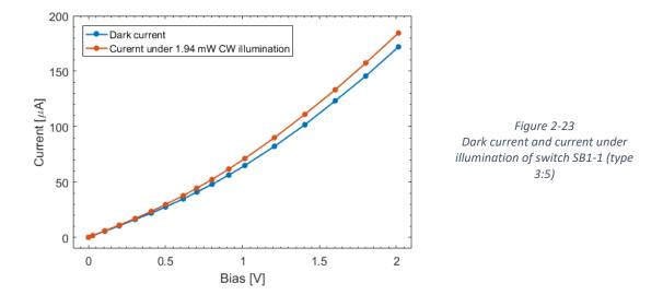
The difference between the dark current and the current under illumination is the photocurrent, which is 6.3  $\mu$ A at 1 V bias, therefore our measured responsivity is 3.24  $\mu$ A/mW which is in the same order as it was measured at UCL.
