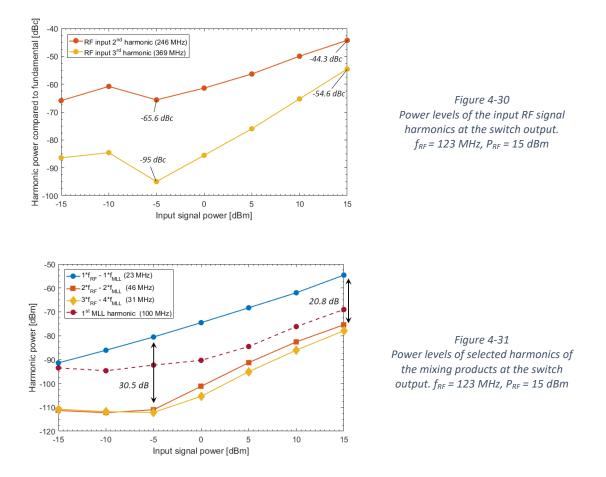
This is showing that while the input signal's second harmonic power changes with 40 dB, the harmonics are changing with only 10 dB, indicating that due to the switch non-linearities high levels of harmonics are also generated from the input  $f_{RF}$  signal.
