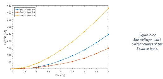
Our measured curves are differing from the one in Figure 2-20 obtained at UCL. The lower level of currents measured by us, indicates the previously obtained higher dark resistance too. These
