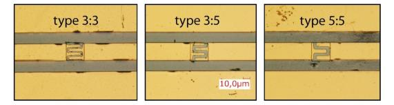
Figure 2-3 Microscope view of the 3 switch types
