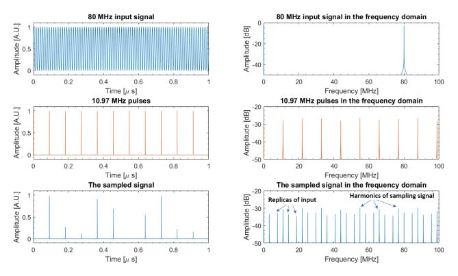
Figure 1-18 Example for undersampling of an 80 MHz sinusoidal signal with 10.97 MHz pulses.
