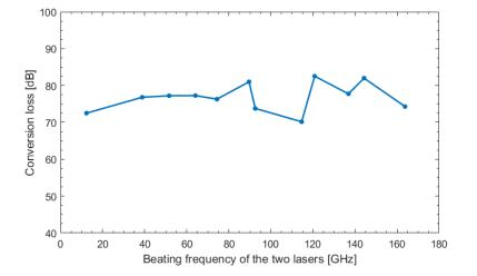
Figure 4-13 Conversion loss of the beating of two DFB lasers versus the beating frequency
