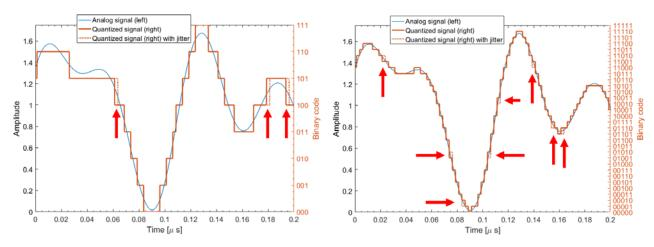
Figure 1-27 Illustration of the jitter effect on the quantized signal for 3 (left) and 5 (right) bits for doubled sampling rate to 400 MHz
