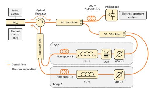
Figure 3-29 Setup of the dual-loop all optical feedback. PC: Polarization controller; VOD: Variable optical delay line; VOA: Variable optical attenuator
