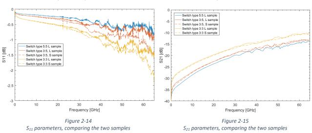
In Figure 2-14 and Figure 2-15 the same types of switches are compared from the two samples, it shows that practically there is no difference between the two samples.
