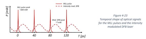
An illustration of the temporal shape of the modulated laser signal is shown in Figure 4-23, it is a sinusoidal with an offset and with a lower peak power than in case of the pulses.
