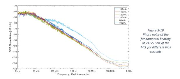
This curve can be converted into the integrated root-mean square (RMS) timing jitter ( $\sigma_{RMS}$ ), which is the standard deviation of the timing accuracy of the signal. It is calculated by the integration of the SSB-PN curve and the result is measured in seconds, as it is used also in [100]:
