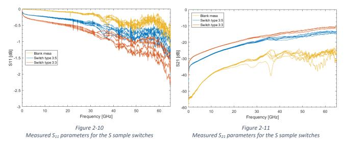
The results show that the feedthrough of the signal is increasing over the frequency and it is also depending on the switch type because the different switches have different capacitances depending on the finger number and gap size.
