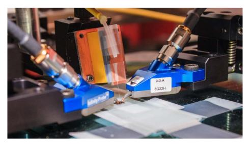
Figure 2-7 Setup on the probe station with two RF probes and the fibre holder
