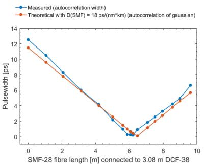
Figure 23 Measured and theoretical pulsewidths for different lengths of SMF-28 fibre plus 3.08m DCF-38, D(SMF)=18, D(DCF)=-38
