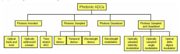
Figure 1-29 Illustration of the photonic ADC categories. Source: G. C. Valley, Optics Express, 2007 [67]
