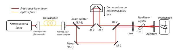
Figure 13 Optical autocorrelation setup with second harmonic generation
