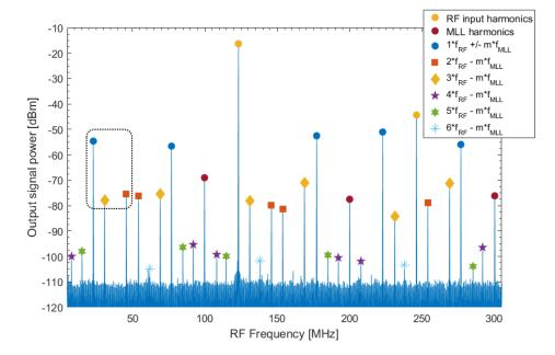
Figure 4-29 RF spectrum of the switch output, Popt=12 dBm, P(RF)=15 dBm. VBW/RBW: 3 kHz/3 kHz
