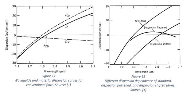
The waveguide dispersion component is dependent on the fibre-design: the core radius (*a*) and the core-cladding index difference ( $\Delta$ ). Changing these properties, the dispersion curve can be shifted to make zero-dispersion fibre at 1.55 µm. Shifting the zero-dispersion point even more, beyond 1.6 µm or more, the  $\beta_2$  will have a large positive value. These fibres are called dispersion compensating fibres (DCF). Figure 12 shows usual dispersion curves for dispersion shifted fibres.
