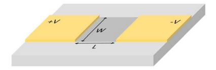
Figure 1-3 Illustration of the photoconductive gap with its dimensions. Usually, these dimensions are in the micrometre range
