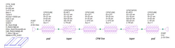
Figure 2-8 Microwave Office model of the CPW waveguides
