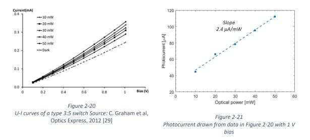
The bias was swept up to 1 Volts. The dark state measurement indicates a closely linear curve, translating it into the dark resistance, its value is around 5.9 k $\Omega \pm 0.3$  k $\Omega$ . An increase in the photocurrent is also observed with increasing optical powers, Figure 2-21 shows the photocurrent by the optical power for 1 Volt bias (*photocurrent = current under illumination - dark current*). The slope gives a responsivity of 2.4  $\mu$ A/mW.
