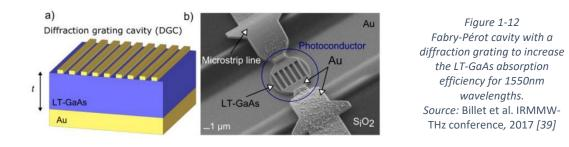
It was shown, that the grating is allowing the excitation of waveguide modes in the structure and increased the efficiency by 3 times. Microwave signal conversion losses of 65 dB was also observed [39].
