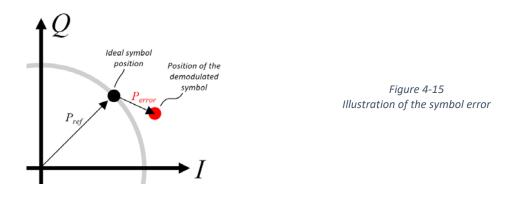
We are recording the EVM percentage for different data-rates of QPSK modulation.
