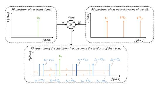
Figure 4-3 Illustration of the mixing products of the proposed mixer scheme
