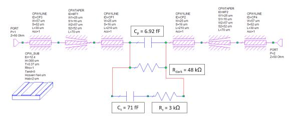
Figure 2-18 Schematics of the improved equivalent model of the photoswitch
