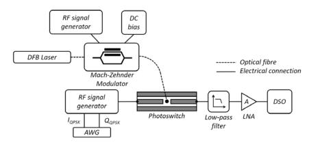
Figure 4-24 Setup for the data-stream downconversion. Intensity modulated DFB laser signal as the local oscillator source
