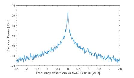
Figure 3-15 Fundamental RF beating signal on a photodiode of the MLL, RBW: 3 kHz, VBW: 5 kHz
