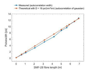
Figure 19 Theoretical and measured 1/e pulsewidths for different length of fibre propagation
