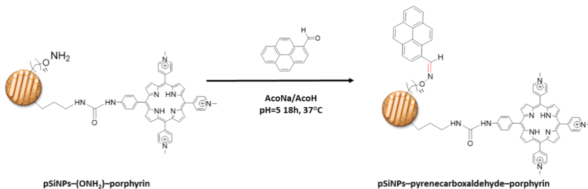
Figure 21. Schematic representation of the 1-Pyrenecarboxaldehyde grafting to obtain pSiNPs-pyrenecarboxaldehyde-porphyrin.
