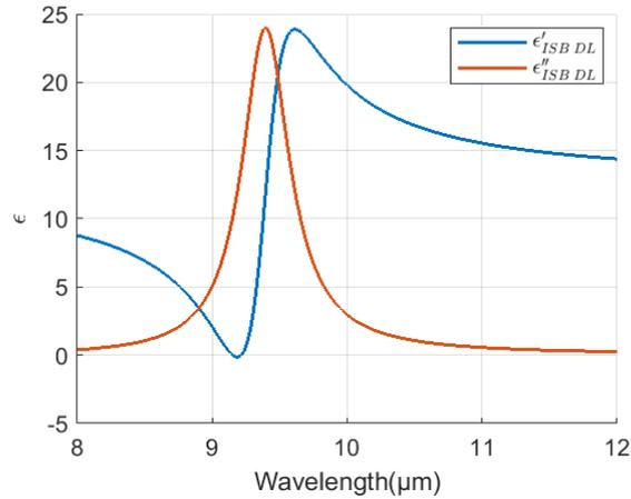
Figure 1.6 – Drude-Lorentz ISB transition dielectric function,  $N=1 \times 10^{18} \text{cm}^{-3}$ ,  $\Gamma_{ISB}=6\text{meV}$ ,  $\epsilon_{\infty}=11.6$
