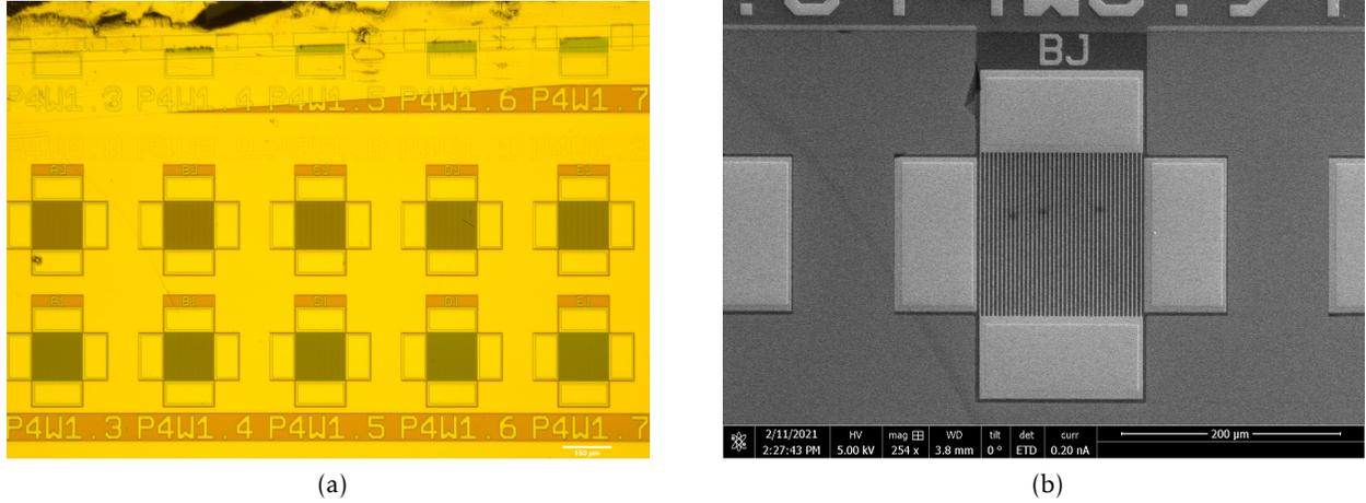
Figure 3.19 – a) Optical and b) SEM images of the devices in TGB4545-6-1. a) depicts the whole array of EOM with different antenna width  $S$ , nominally varying from  $0.8$  to  $1.7\mu\text{m}$ , incremented by  $0.1\mu\text{m}$  each. b) shows the complete structure of an EOM.
