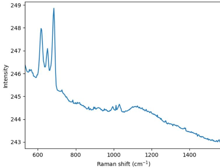
Figure 2.18 – Raman measurement of plasmon-phonon coupling in n-doped InGaAs. A broad peak at about  $1117\text{cm}^{-1}$  is assigned to the  $L_+$  mode. The corresponding electron density is about  $1.325 \times 10^{19}\text{cm}^{-3}$ . Other sharper peaks at around  $650\text{cm}^{-1}$  are assigned to higher harmonic of InP phonons ( $\omega_{LO} \sim 344\text{cm}^{-1}$ ,  $\omega_{TO} \sim 303\text{cm}^{-1}$  [28]).
