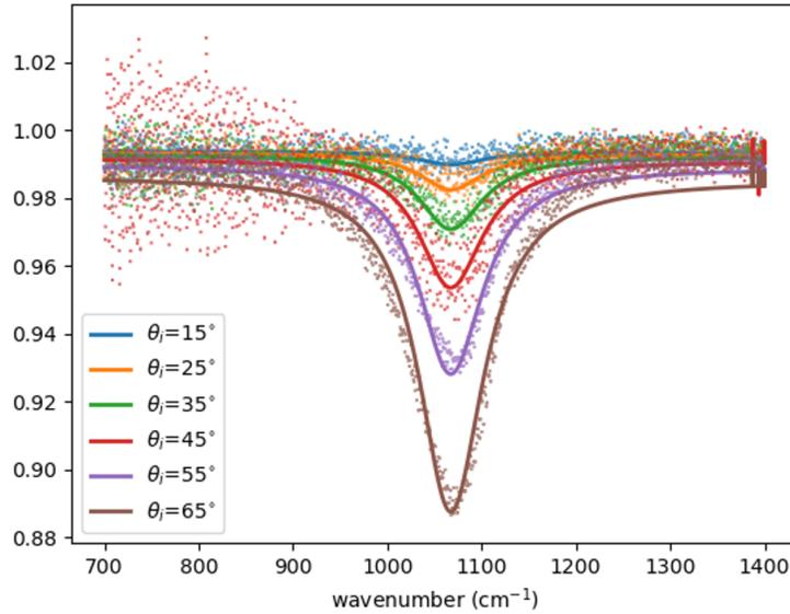
Figure 2.19 – FTIR reflectance measurement of TGB4545-2-1, transferred on gold substrate. A dip at about  $1070\text{cm}^{-1}$  which becomes deeper at larger incident angle is assigned to the Berreman mode in InGaAs layer. We can deduce a doping of about  $1.24 \times 10^{19}\text{cm}^{-3}$  in the layer and a damping factor  $\Gamma \sim 71.9\text{cm}^{-1}$ .
