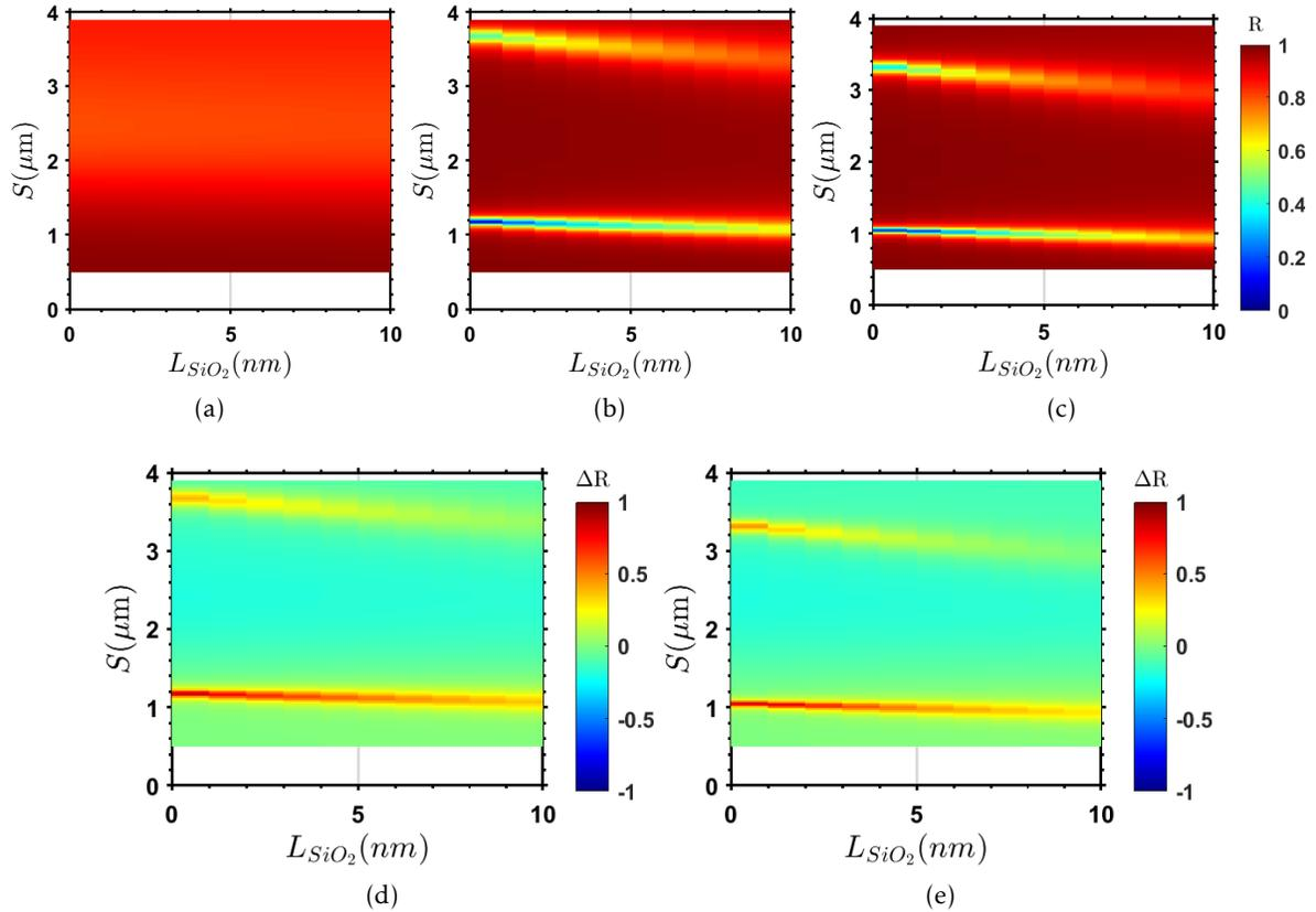
Figure 3.26 – a, b, c) Reflectance map of MOSFET-like ENZ-EOM structure at different electron concentrations, normal incidence: a)  $N=1.3 \times 10^{19} \text{cm}^{-3}$ , b)  $N=5 \times 10^{18} \text{cm}^{-3}$ , c)  $N=0 \text{cm}^{-3}$ . a, b, c) share the same color scale. d, e) Modulation amplitude maps between the strong coupling regime  $N=1.3 \times 10^{19} \text{cm}^{-3}$  and two depletion regimes  $N=5 \times 10^{18} \text{cm}^{-3}$  in d) and  $N=0 \text{cm}^{-3}$  in e).
