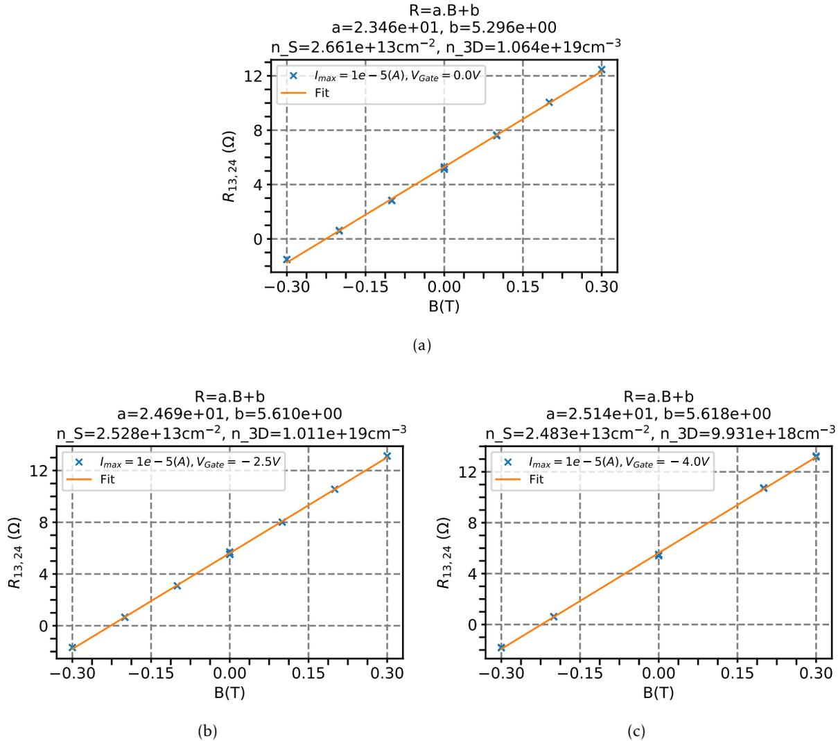
Figure 3.35 – Hall effect Van der Pauw measurements under bias Grid-Back contact a) Zero bias, b) -2.5V bias, c) -4V bias. The 3D electron density at 0V bias is about  $1.06 \times 10^{19} cm^{-3}$ . At -4V, the electron concentration is reduced to  $0.99 \times 10^{19} cm^{-3}$ , representing a reduction by about 7% of the total electron density.
