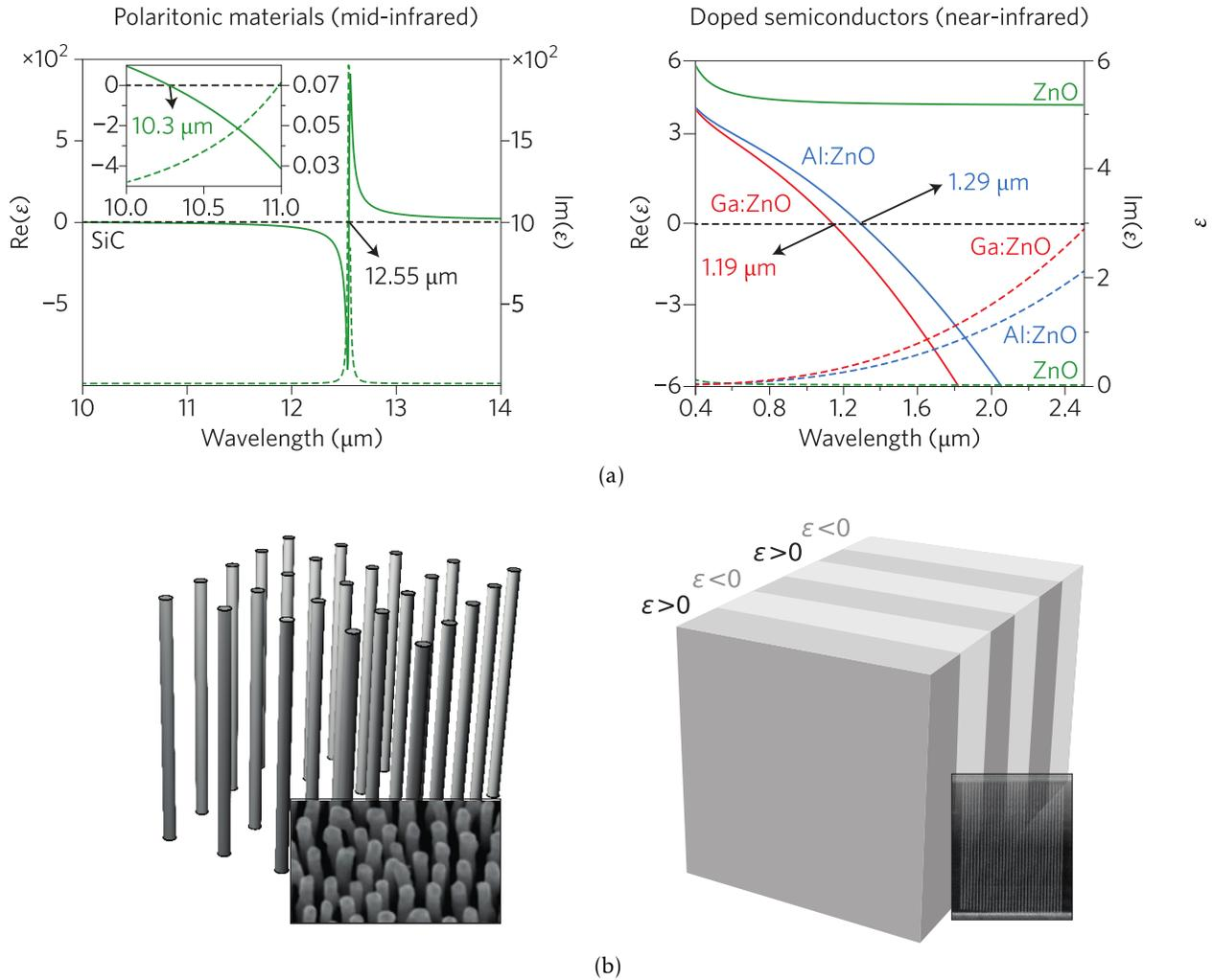
Figure 1.2 – ENZ materials: continuous and inhomogeneous media, figure adapted from reference [18]. Top figures illustrate the dielectric functions of continuous ENZ media: Phononic materials SiC,  $\lambda_{ENZ} \sim 10.3\mu\text{m}$ ; doped oxide ZnO,  $\lambda_{ENZ} \sim 1.3\mu\text{m}$ . Bottom figures illustrates inhomogeneous ENZ media: metallic nanorods (gold) in dielectric medium (air); metallic-dielectric multilayer made of Ag-SiN
