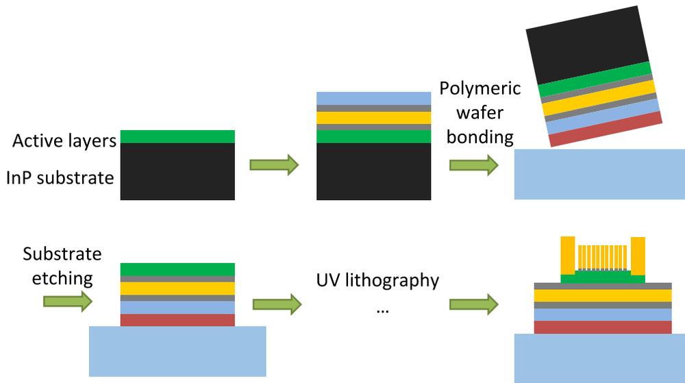
Figure 3.17 – Steps of the fabrication process.
