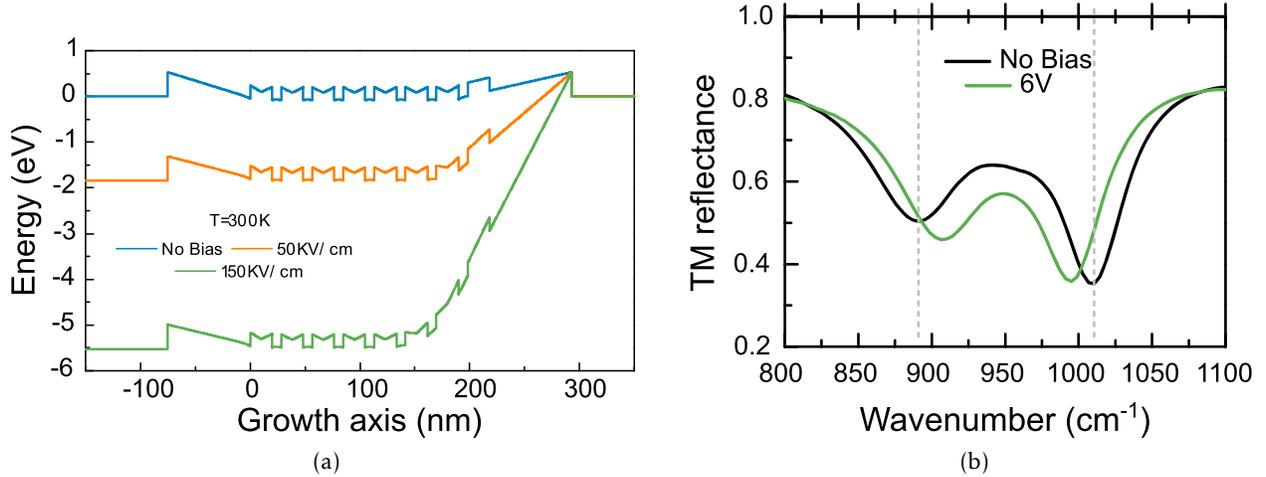
Figure 3.4 – Adapted from reference [3]. a) Band structure of the modulator at different bias regimes. b) Reflectance spectra change between two regimes.
