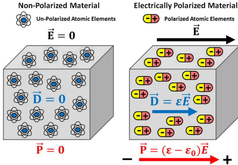
Figure 1.1 – Material’s polarization under external electric field [5]
