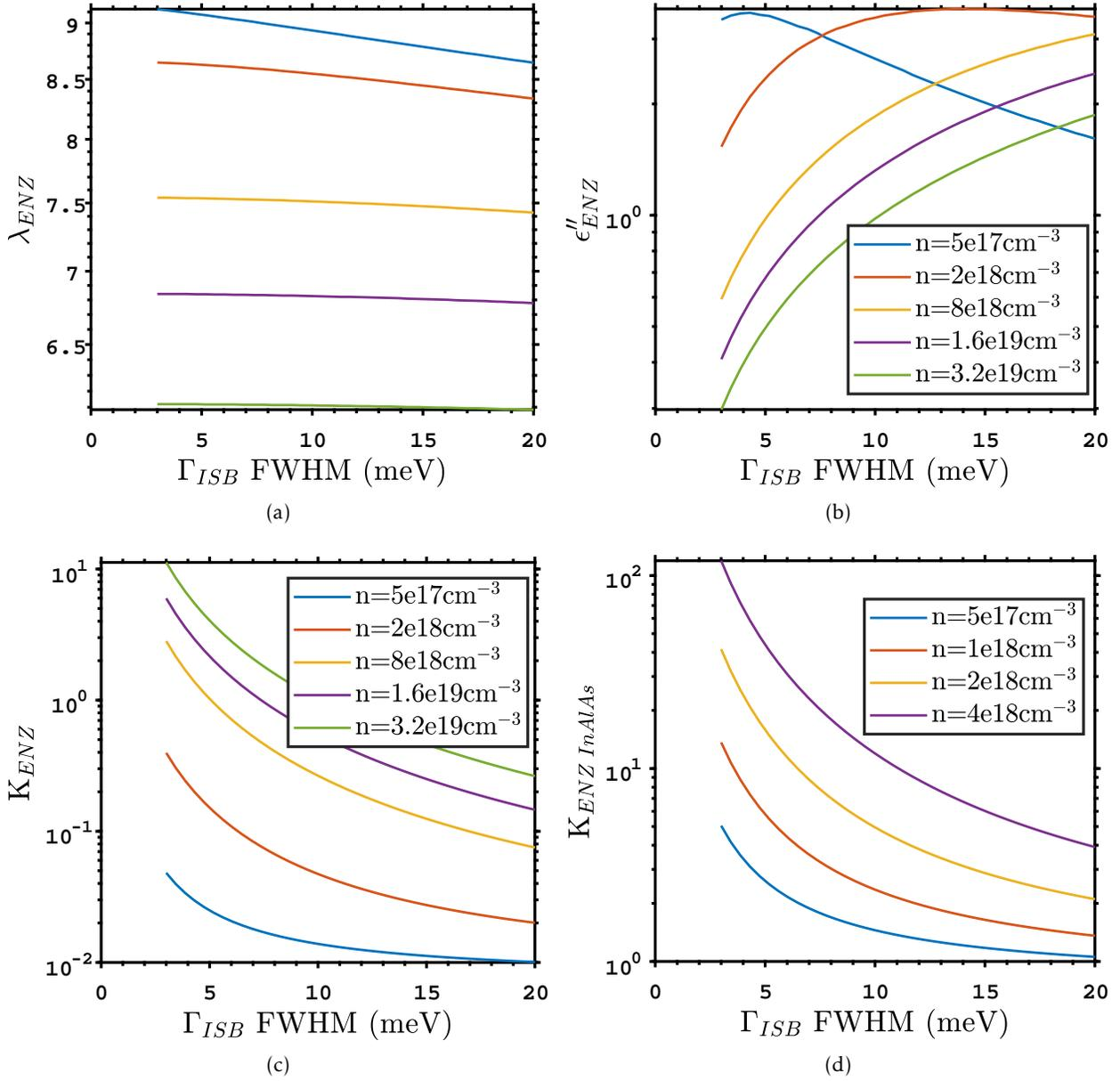
Figure 2.21 – (a)  $\lambda_{ENZ}$ , (b)  $\epsilon''_{ENZ}$ , (c)  $K_{ENZ}$ , (d)  $K_{ENZ InAlAs}$  computed with different dopings and damping factors using DL model. a), b) and c) share the same legend for curves.
