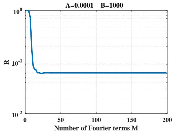
Figure 3.10 – Convergence test of reflectance of a metallic grating structure as a function of the number of Fourier terms.
