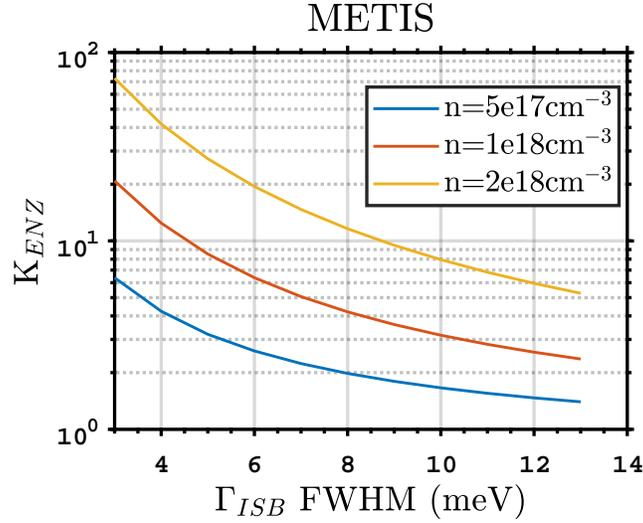
Figure 4.6 –  $K_{ENZ InAlAs}$  computed with different dopings and damping factors using METIS data. For  $N=1 \times 10^{18} \text{ cm}^{-3}$ ,  $K_{Dielectric InAlAs} \sim 2.7$  for  $\Gamma_{ISB}=12 \text{ meV}$  and  $K_{ENZ InAlAs} \sim 6.5$  for  $\Gamma_{ISB}=6 \text{ meV}$ .
