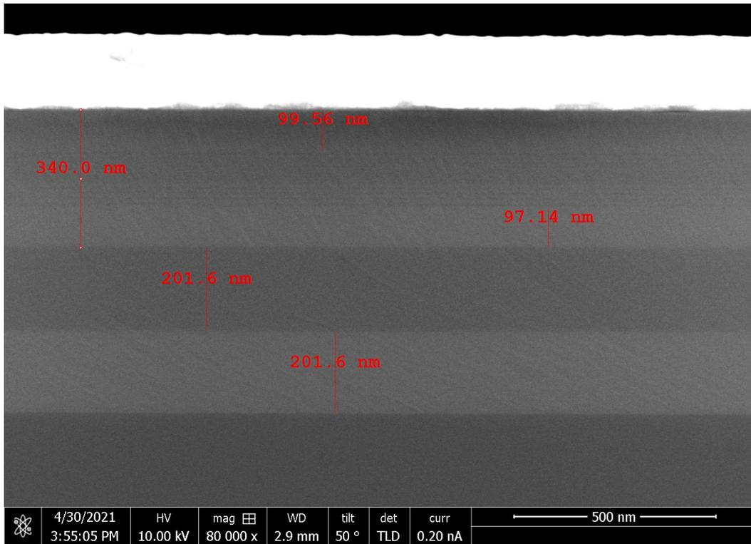
Figure 40 – SEM image of QCD40 substrate’s cross section with Ti/Au/Ti/SiO<sub>2</sub>/Ti on top.
