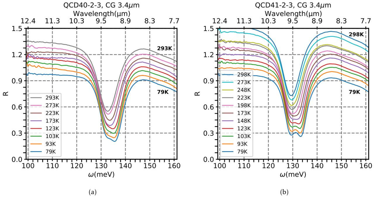
Figure 4.18 – a) and b) Reflectance spectra at different temperatures of device 'CG', whose  $S=3.4\mu\text{m}$  nominally. Each spectrum is offset by 0.05 from the previous one. We observe the appearance of the ISB absorption peak when the temperature decreases from room temperature down to 79K.
