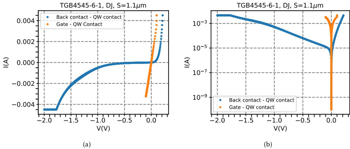
Figure 3.22 –  $I(V)$  characteristic of HEMT-like EOM.  $I(V)$  Back contact - QW contact (blue line) shows a Schottky diode behavior whereas  $I(V)$  Gate - QW Contact (orange line) shows an Ohmic behavior. a) Linear scale plot, b) Semilog scale plot of the same data.
