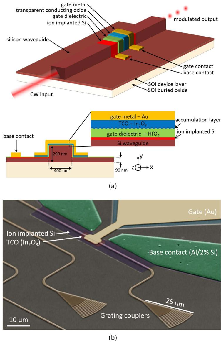
Figure 3.2 – Adapted from reference [11]: a) schematic of an ENZ-EOM with In<sub>2</sub>O<sub>3</sub> as ENZ layer on Si waveguide. b) SEM image of the experimental device.
