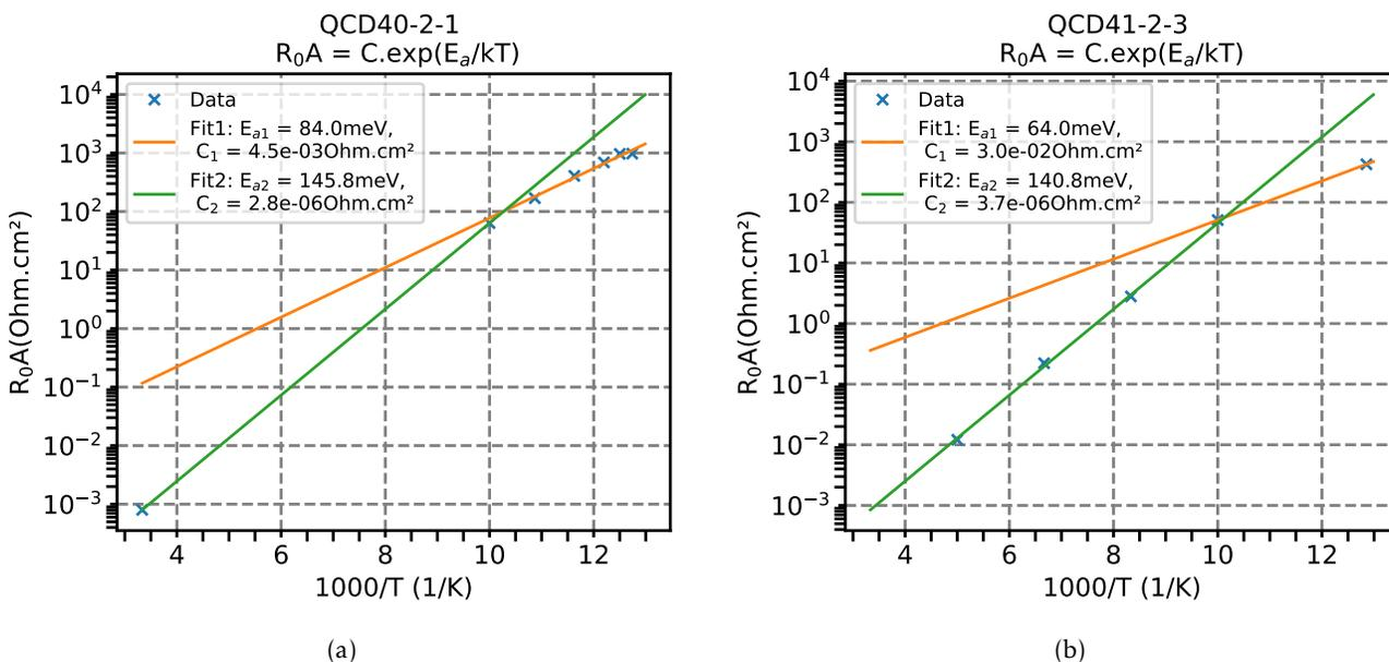
Figure 4.22 – Fitting of  $R_0A$  with the relation  $R_0A=C.exp(E_a/kT)$  for two sets of data:  $1000/T > 10K^{-1}$  ( $T < 100K$ , orange line) and  $1000/T < 10K^{-1}$  ( $T > 100K$ , green line). a) QCD40-2-1:  $E_{a1} = 84.0meV$ ;  $E_{a2} = 145.8meV$ . b) QCD41-2-3:  $E_{a1} = 64.0meV$ ;  $E_{a2} = 140.8meV$ .
