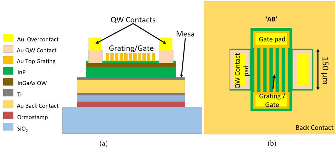
Figure 3.16 – Final structure of EOM: a) side view, b) top view. Optically, the active structure is located under the grating zone, with an area of  $150 \times 150 \mu\text{m}^2$ . Electrically, the device consists of three electrical terminals: the top gate, the QW contact and the back contact.
