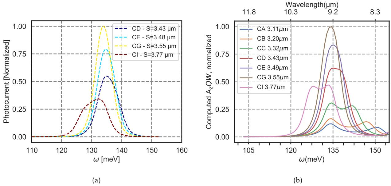
Figure 4.39 – a) Computed photocurrent spectra with CMT, giving relative amplitudes between different devices. b) Computed useful  $A_z QW$  for different devices with Reticolo, normalized to the maximum of  $A_z CG$ .
