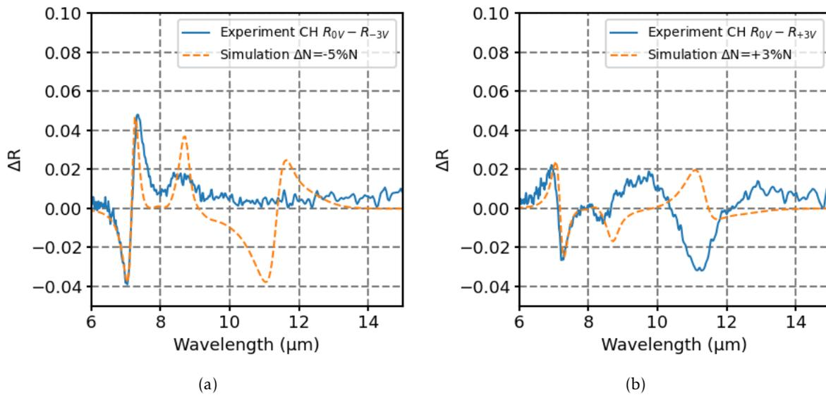
Figure 3.41 – Comparison between the experimental modulation amplitude of the device 'CH' ( $S_{exp}=1.167\mu\text{m}$ ) and the simulation. a) A negative bias of -3V in experiment and a reduction of 5%N of the electron density in the QW in simulation. b) A positive bias of +3V in experiment and an increase of 3%N of the electron density in the QW in simulation. Good agreement between experiment and simulation is observed around the peak A but not around the peaks B and C.
