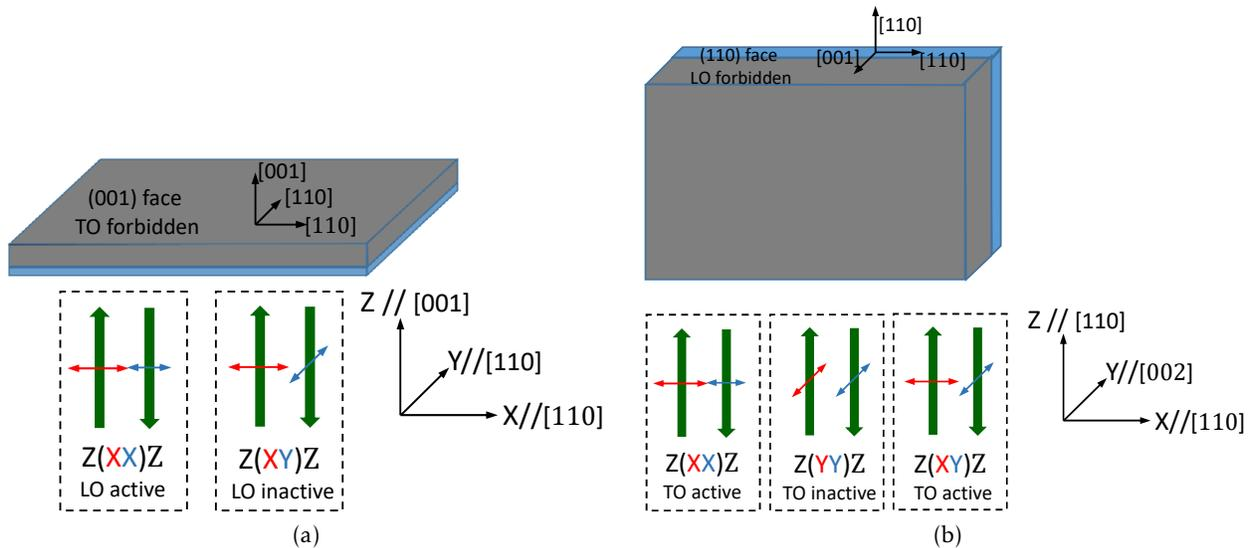
Figure 2.4 – Raman selection rule for zinc-blende structure.
