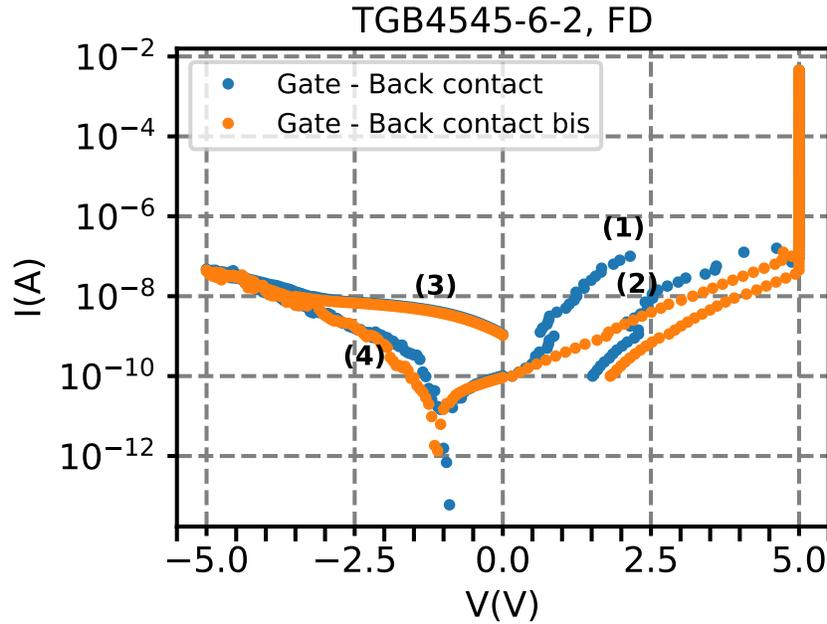
Figure 3.34 –  $I(V)$  characteristic of MOSFET-like EOM TGB4545-6-2:  $I(V)$  Gate-Back Contact show an insulator behavior, with hysteresis. Forward  $V(I)$  scan starts at  $I=10^{-10}$  A. The order of the scan is indicated by numbers (1), (2), (3), (4) for the blue curve.
