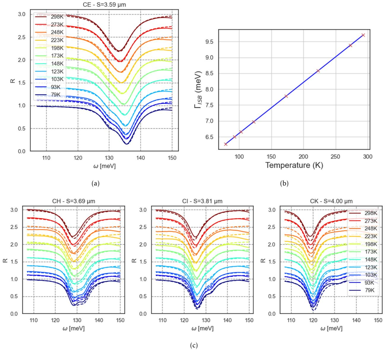
Figure 4.34 – a) Data fitting with CMT of reflectances with 'CE' dataset of sample QCD41-2-3. b) Evolution of  $\Gamma_{ISB}$  as a function of temperature. c) The obtained parameters are used to compute the reflectance spectra of 'CH', 'CI', 'CK'.
