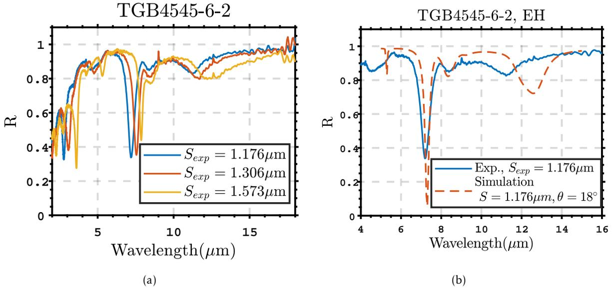
Figure 3.33 – a)  $\mu\text{FTIR}$  measurement with floating bias. A strong absorption at around  $7\mu\text{m}$  two weaker peaks at around  $8$  and  $12\mu\text{m}$  correspond to the coupling between MIM mode, InGaAs free charges ENZ mode and  $\text{SiO}_2$  phonon ENZ mode. b) Experimental and simulated reflectance spectra with  $S_{exp} = 1.176\mu\text{m}$ , Au Ordal.
