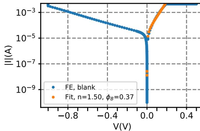
Figure 3.23 – Diode model fitting of TGB4545-5-1 FE
