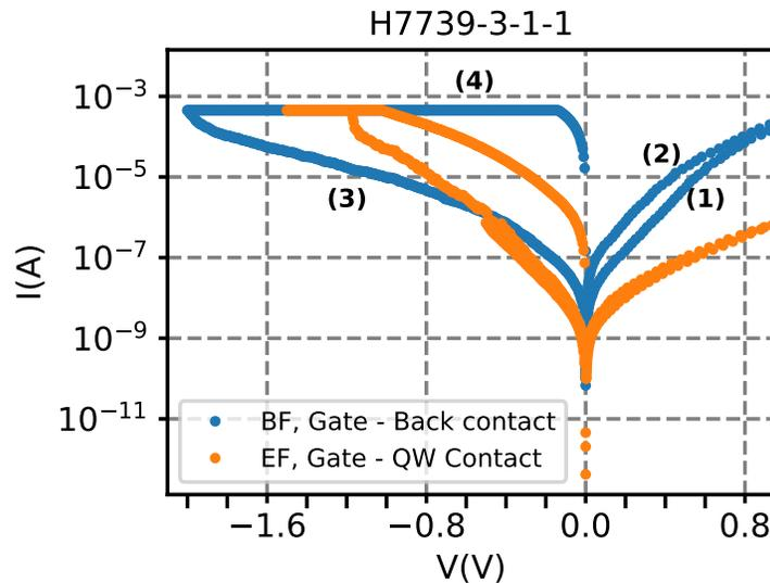
Figure 3.30 –  $I(V)$  characteristics of H7739-3-1-1 with 5nm of  $\text{SiO}_2$  sputtering as insulator. Forward  $V(I)$  scan starts at  $I=10^{-10}$  A. The order of the scan is indicated by numbers (1), (2), (3), (4) for the blue curve.
