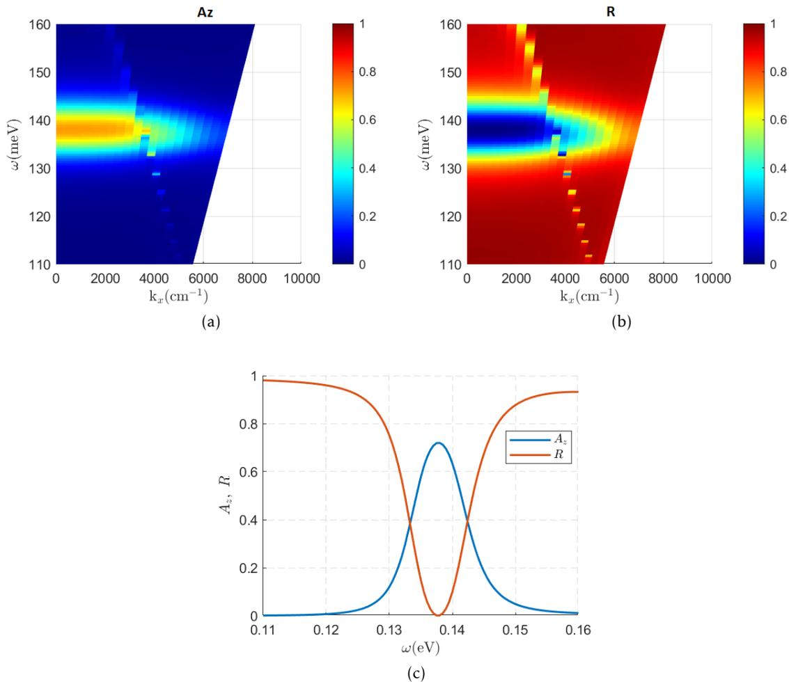
Figure 4.9 – Computation with Reticolo: a,b) Useful absorption  $A_z$  and reflectance  $R$  of QCD. c) Absorption  $A_z$  and reflectance  $R$  spectra at normal incidence. Ordal dielectric functions for Au, Ti.
