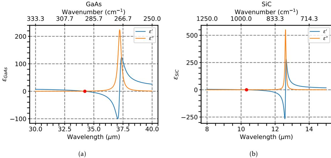
Figure 1.9 – Contribution of optical phonons to the dielectric function in GaAs (left) and SiC (right). The red dots indicate the zero crossing of  $\epsilon'$ , respectively at  $34.2\mu\text{m}$  and  $10.3\mu\text{m}$  for intrinsic GaAs and SiC.
