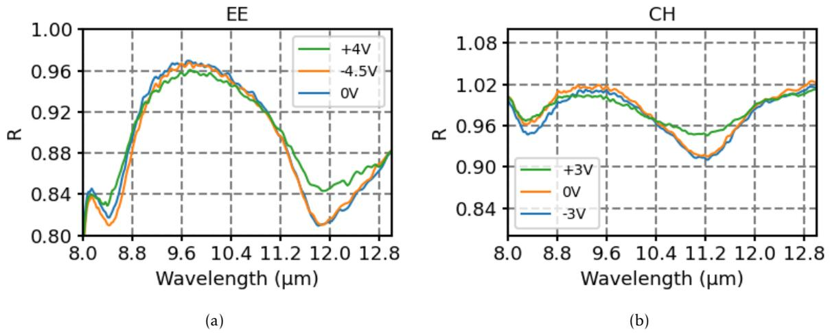
Figure 3.40 –  $\mu\text{FTIR}$  measurement under bias. Two absorption peaks at  $8.5\mu\text{m}$  (B) and  $12\mu\text{m}$  (C)
