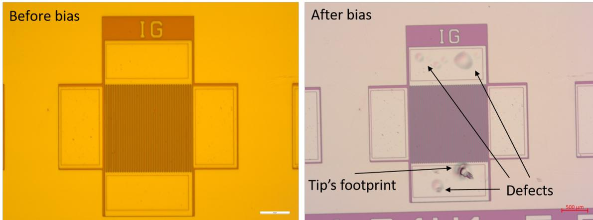
Figure 3.42 – The device before and after high bias voltage ( $-4V$ ) application. Some bubble-like defects appear on the top gate pads.
