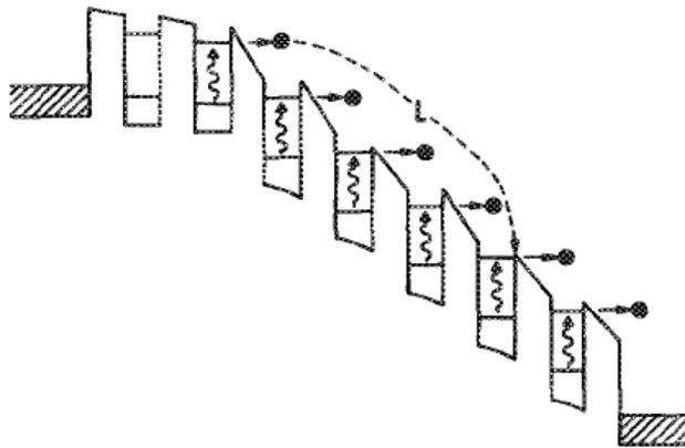
Figure 4.1 – QWIP’s band structure under bias, adapted from reference [111] - the first demonstrated QWIP. The device is a photoconductive detector, made of a repetition of identical GaAs/AlGaAs n-doped quantum wells. Using bound-to-bound configuration, under illumination, an electron is promoted to the excited state by photon absorption, then tunnels out of the QW into the continuum, creating a photocurrent.
