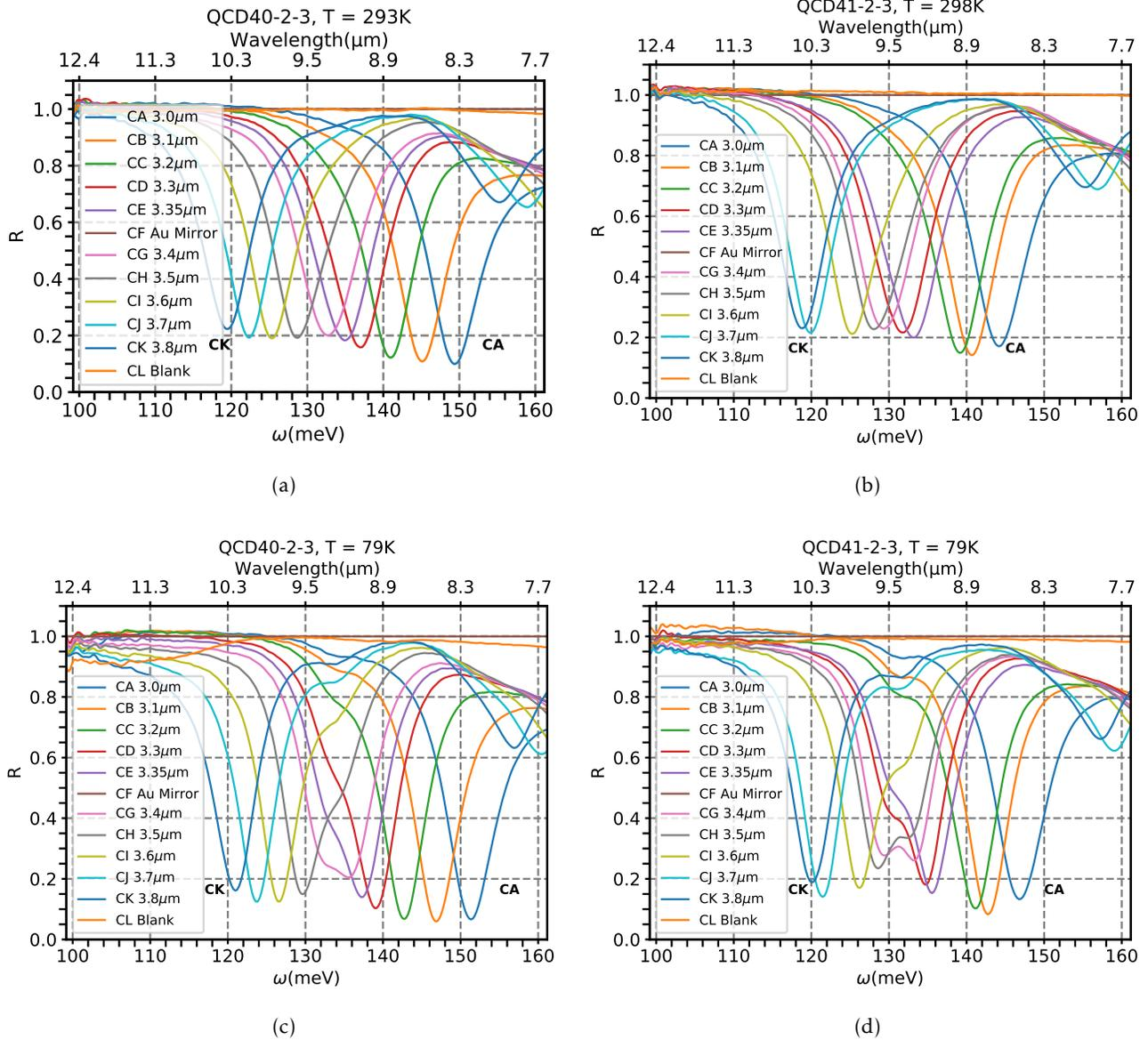
Figure 4.15 – a) and b) Reflectance spectra of devices with various strip width  $S$  on samples QCD40-2-3 and QCD41-2-3 at room temperature. The reflectance dip amplitude becomes shallower and the absorption linewidth increase towards 'CG' device. This is a sign of the ISB transition in the QCD structure at room temperature.
