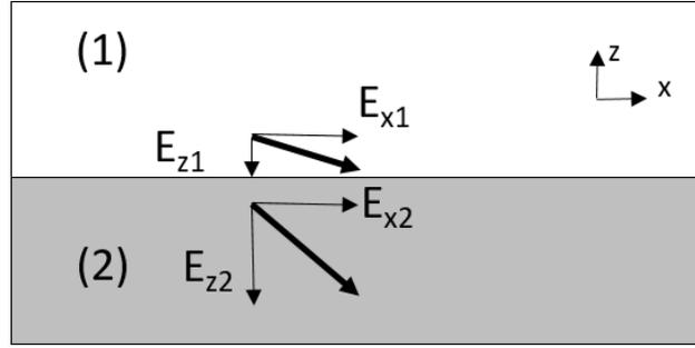
Figure 1.3 – Interface between two media (1) and (2)
