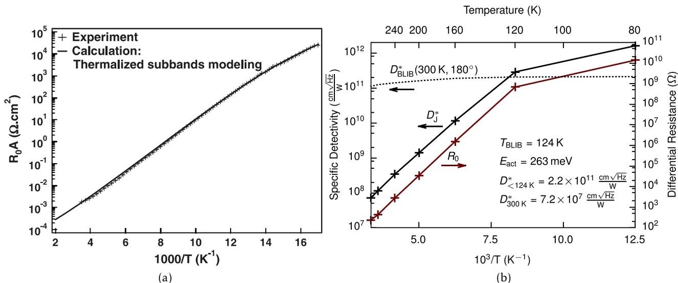
Figure 4.23 – a) Adapted from reference [116]:  $R_0A$  measurement and computation (with thermalized subbands model) for a QCD device operating at  $8\mu\text{m}$ , having 10 periods with doping  $3.5 \times 10^{11} \text{ cm}^{-2}$  for each active QW.  $R_0A(1000/T)$  curve in a) behaves quite similarly and having  $R_0A$  of the same order of magnitude with samples QCD40-2-1, QCD41-2-3 (Figure 4.22b).
