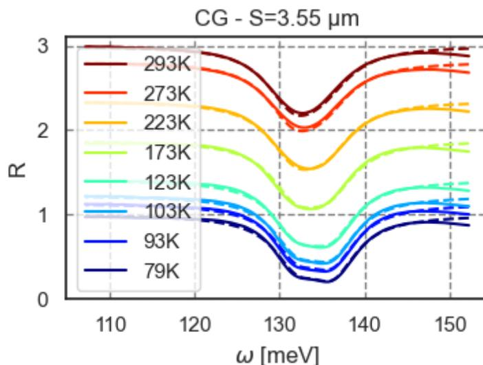
Figure 4.36 – Data fitting with CMT of reflectances with 'CG' dataset of sample QCD40-2-3.
