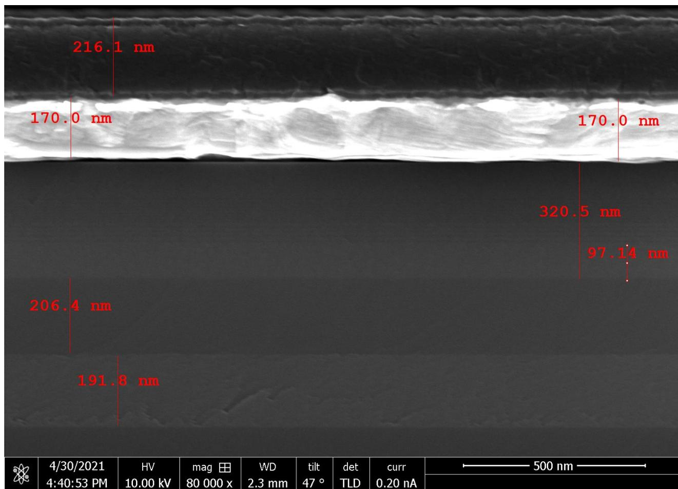
Figure 4.11 – SEM image of QCD41 substrate’s cross section with Ti/Au/Ti/SiO<sub>2</sub>/Ti on top. The one of QCD40 is given in Appendix B.3.
