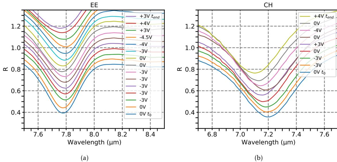
Figure 3.37 –  $\mu$ FTIR measurement under bias. Devices: 'EE'  $S_{exp}=1.486\mu\text{m}$ , CH  $S_{exp}=1.176\mu\text{m}$ . The spectra are shifted by  $+0.05$  each time in the chronological order of data acquisition, starting from  $t_0$  (bottom) to  $t_{end}$  (top). A small but reproducible optical modulation is observed in the reverse bias regime (both 'EE' and 'CH'). The irreversible behavior is observed in 'CH' in the forward bias regime.
