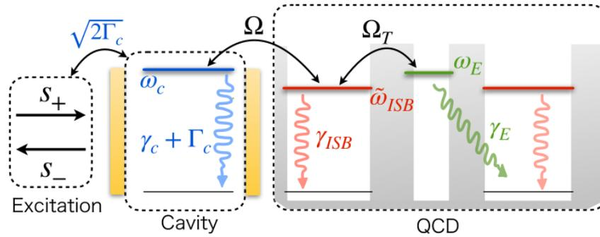
Figure 4.33 – Schematic of CMT with a three-resonator system in QCD, adapted from reference [117].
