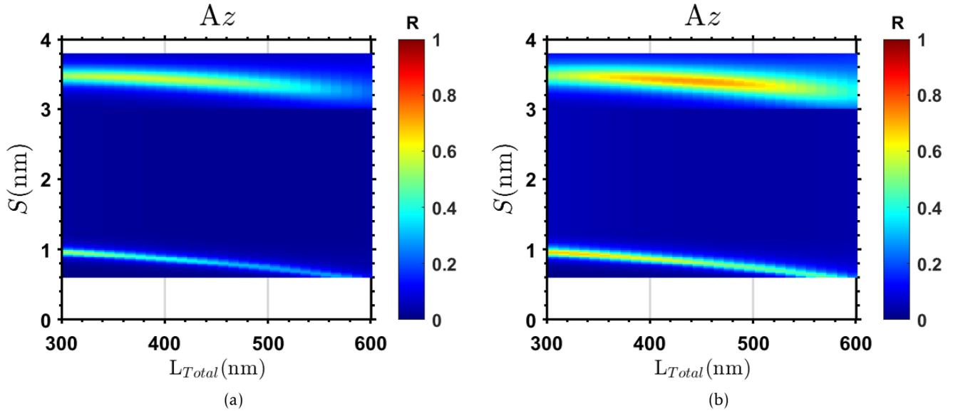
Figure 4.7 – Computation with Reticolo: Optimization of  $A_z$  QW as a function of strip’s width  $S$  and total semiconductor thickness  $L_{total}$ . The period  $P$  is fixed at  $6\mu\text{m}$ . The doping concentration of the QW is  $5\times 10^{17}\text{cm}^{-3}$  in a) and  $1\times 10^{18}\text{cm}^{-3}$  in b).
