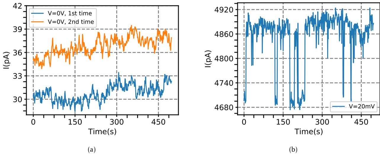
Figure 4.24 – Evolution of dark current as a function of time of a device on QCD40-2-1, integration time 1s per data point: a)  $V=0V$ , mean value of  $I$  31-36pA and standard deviation of  $I$  1.1pA. b)  $V=20mV$ , mean value of  $I$  4850pA and standard deviation of  $I$  64pA.
