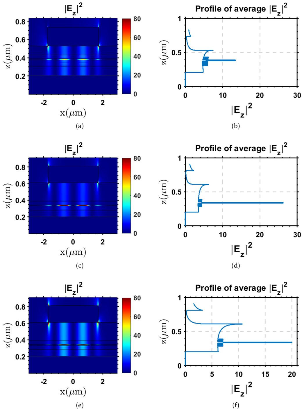
Figure 4.32 – Left:  $|E_z|^2$  distributions. a) and c) are computed respectively for optimized structure of QCD40 and QCD41 with updated parameters of dielectric function of Au ( $\omega_p = 8.5eV$ ,  $\Gamma = 0.71eV$ ) and the ISB transition ( $\Gamma_{ISB} = 6.5meV$ ). e) is the initial optimization computed for QCD41, with Au dielectric function of Ordal and  $\Gamma_{ISB} = 12meV$ .
