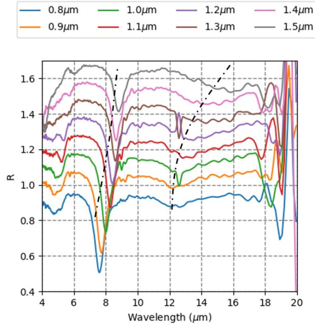
Figure 3.21 –  $\mu$ FTIR reflectance measurement at zero bias. Reflectance of devices with various strip width  $S$  (nominal values), increasing from 0.8 to 1.5  $\mu\text{m}$  by step of 0.1  $\mu\text{m}$ , on sample TGB4545-6-1.  $R$  values are offset for clarity. Anti-crossing of MIM mode and ENZ mode is observed. Two dashed-dotted black lines are added, connecting the peak positions, to guide the eyes.
