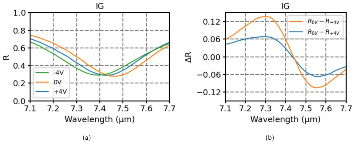
Figure 3.39 – a)  $\mu$ FTIR measurement under bias. Devices: 'IG'  $S_{nominal}=1.5\mu\text{m}$ . The amplitude of modulation is about 0.10 (or 1.2dB of modulation depth). The device shows an irreversible behavior after positive bias.
