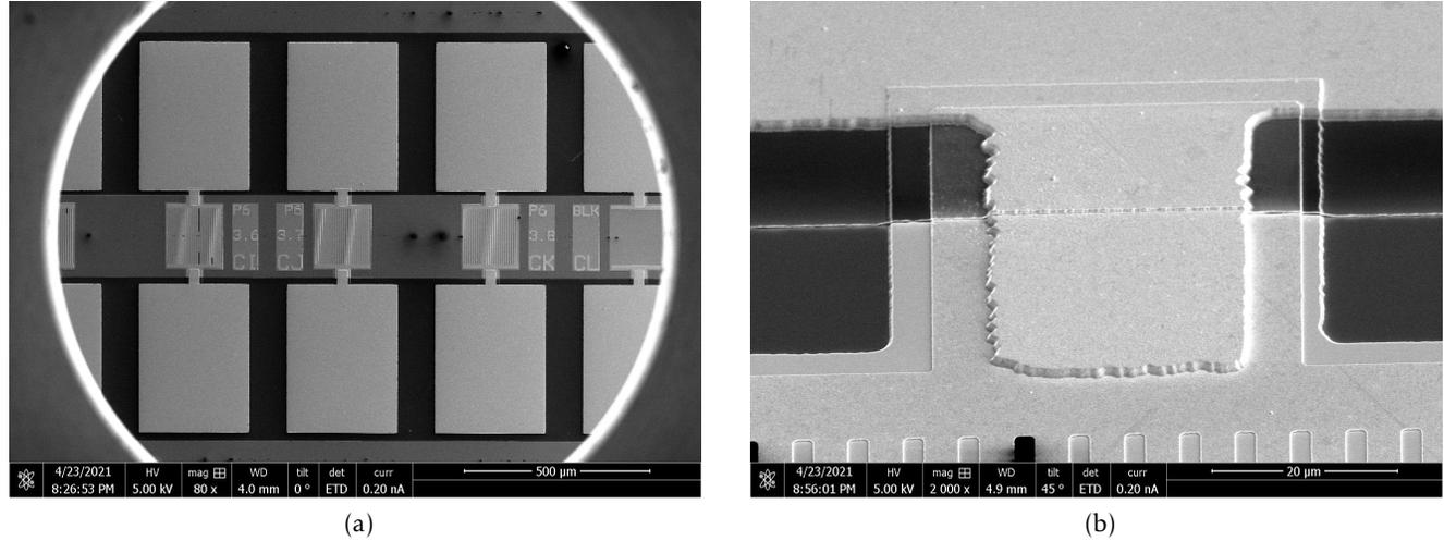
Figure 4.13 – SEM images of QCD devices and contacts levels.
