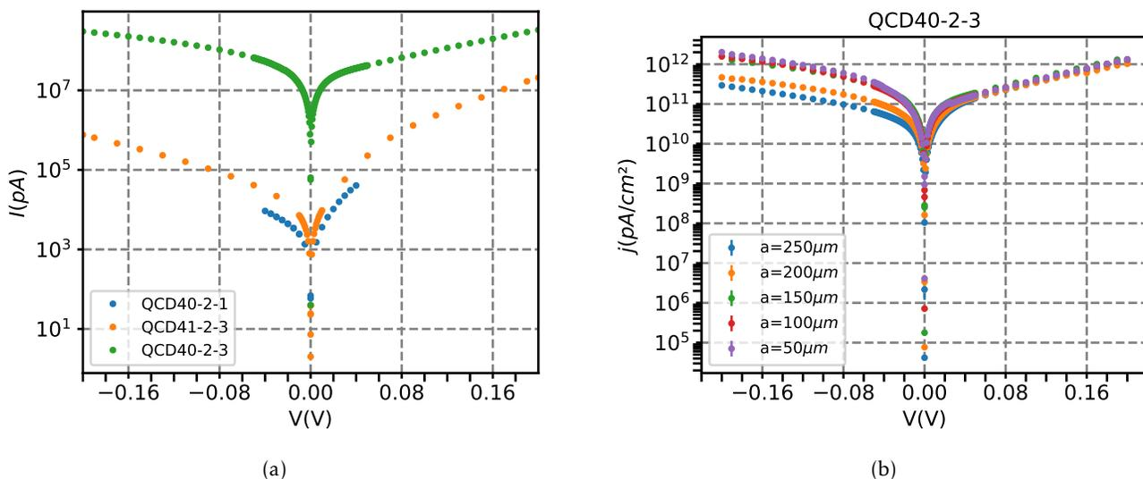
Figure 4.20 – a)  $I(V)$  at 78K in dark of three devices on samples QCD40-2-1, QCD41-2-3, QCD40-2-3. We observe a rectifying behavior for QCD40-2-1, QCD41-2-3 in the expected direction, whereas QCD40-2-3 presents a rectifying behavior in the opposite direction.
