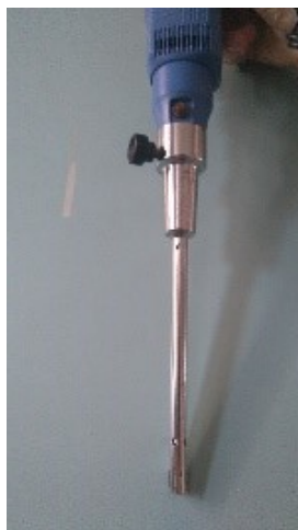
Figure II. 2: Mixing device for NMP slurries (Ultraturax).
