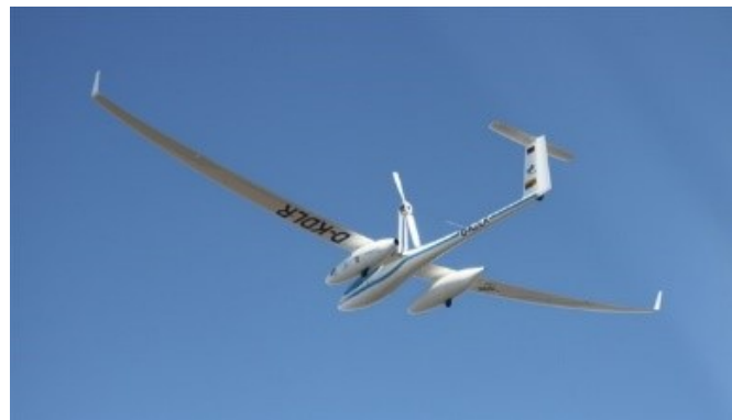
Figure I. 5: Picture of Antares DLR-H2 the first aircraft powered by fuel cells (source: https://www.dlr.de ).
