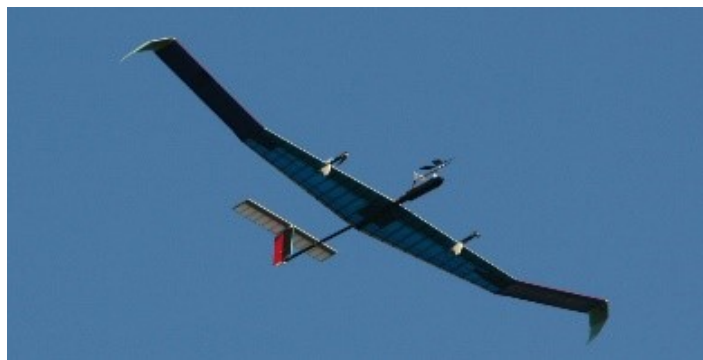
Figure I. 4: Picture of Zephyr 7, the Airbus drone powered by photovoltaic cells and Li-sulfur cells (source: https://www.droneuniversities.com ).
