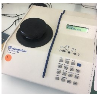
Figure II. 18: Picture of the pycnometer (AccuPyc 1330, Micromeritics).
