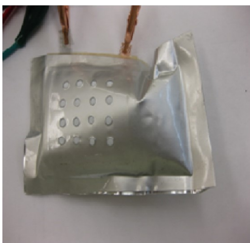
Figure I. 36: Picture of a Li-air pouch cell with gas diffusion membrane (PTFE) after discharge in ambient air. 186
