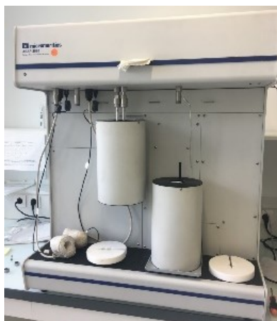
Figure II. 19: Picture of the N_2 adsorption and desorption measurement device at 77 K using N_2 (ASAP 2020, Micromeritics).
