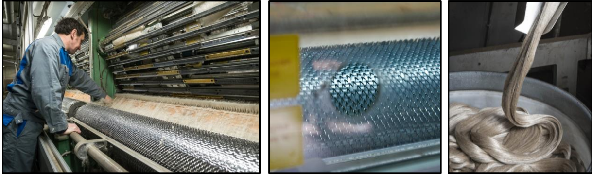
Figure I-13: Hackling operation with the obtention of a continuous ribbon of flax fibres (reprinted with permission from the following sources: https://www.embrin.fr/ ; https://blog.libecohomestores.com/fr/metier-de-lin-fr/extraire-la-fibre/ ).
