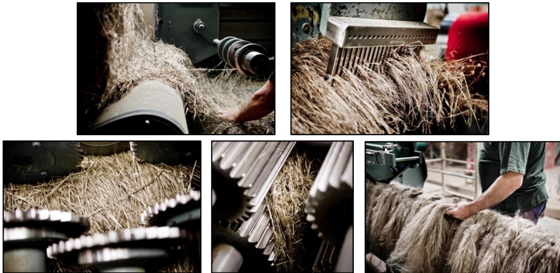
Figure I-12: Different operations present on the scutching line (reprinted with permission from the following source: https://blog.libecohomestores.com/fr/metier-de-lin-fr/extraire-la-fibre/ ).
