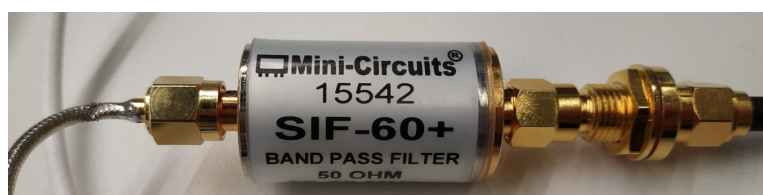
Figure 5.15: Band-pass filter placed after the first LNA.
