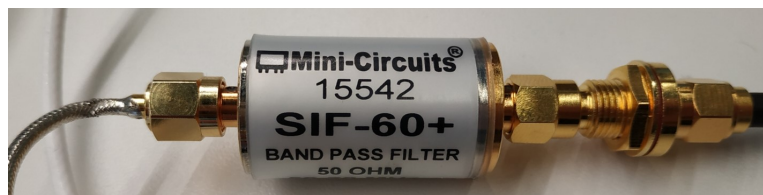
Figure 5.15: Band-pass filter placed after the first LNA.
