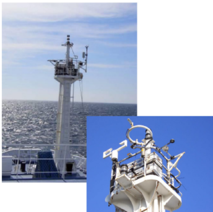
Figure 2.3: CSASP sensors and wind sensors mounted at the top of the R/V Atalante foremast during the MIRAMER campaign. A CSASP-100-HV-ER probe is placed above a CSASP-200 probe.
