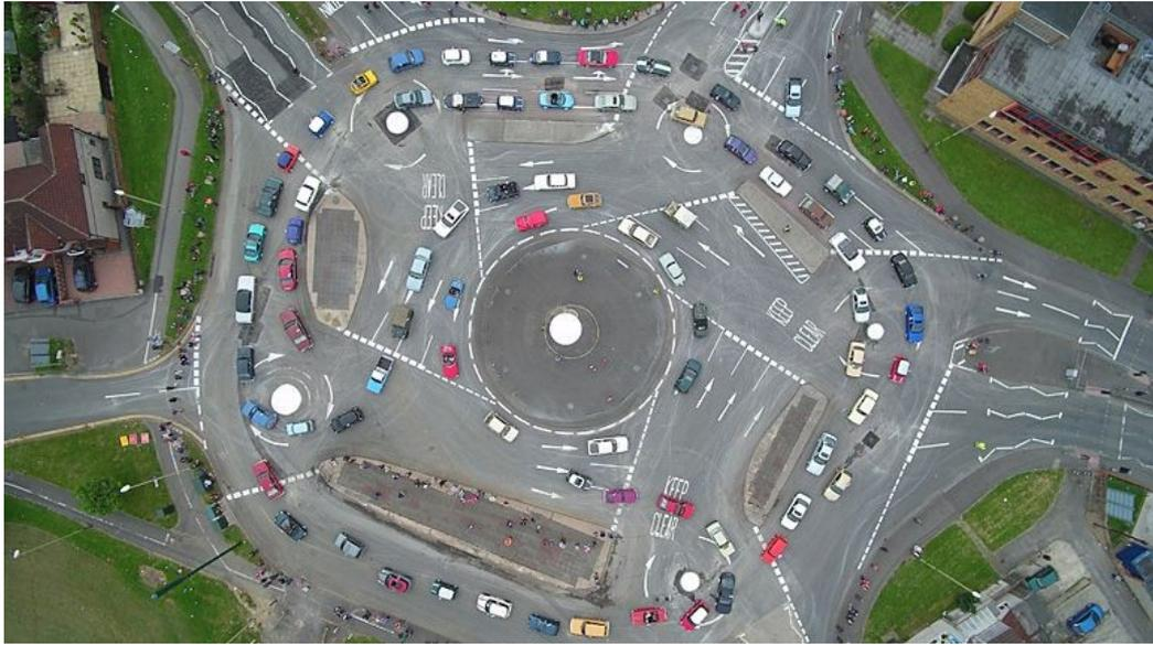
Figure 1.11: Complex roundabout; source Wadman (2017)
