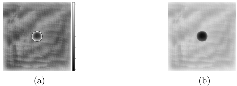
Figure 3.41: An example of a phase unwrapped by means of a guided path following method. (a) Original phase. (b) Unwrapped image.
