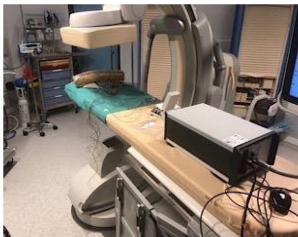
Fig.108: Overview of the experiment. The spinal custom model is positioned in the X-ray beam of a CBCT suite. The DEA generator is positioned on the examination table.
