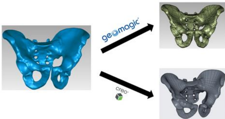
Fig.54: Creation of a solid version of the bone structure from the meshwork of the STL file using two different softwares ([Harrer 2020]).
