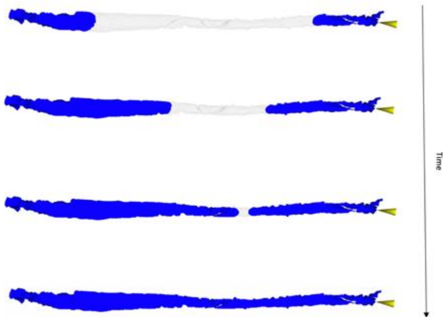
Fig.7.1: progressive filling of the mold by cement (in blue) from both injection points (humerus2). ([Anselmini 2020])
