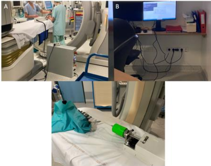
Fig.128: Robotic injection of a large volume of cement. (A) Installation of the robot and the computer in the CBCT suite. (B) Remote control of the robot. (C) Overview of the robot. The sheath surrounded by the eutectic gel is plugged to the piston on one side and to the bone trocar on the other side
