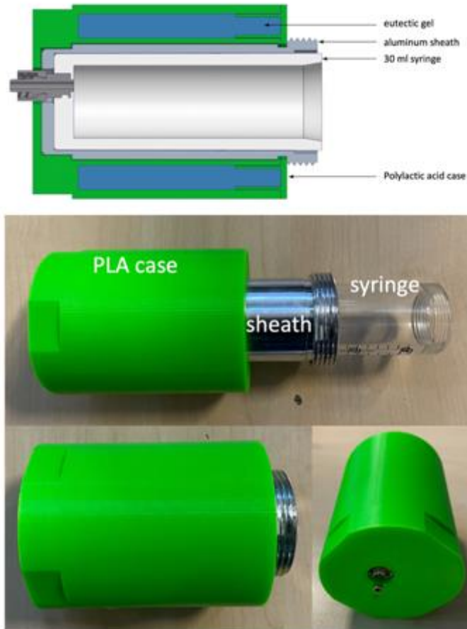
Fig.126: Design of the PLA case filled with eutectic gel to ensure cooling of the aluminum sheath
