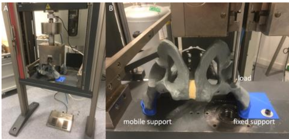
Fig.47: Set-up for the compressive test. (A) Overview of the installation. (B) Magnified picture showing the normal pelvic model with both iliac crests fixed in their corresponding support. The one on the side of the test is fixed. Compression load is applied vertically on the acetabular roof.
