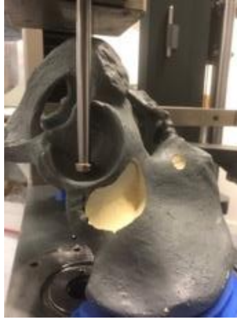
Fig.48: Test for the large tumor model filled with 20% of cement. The lateral view demonstrates the axis of the applied load.
