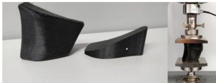
Fig.87: Compression test. A 3D printed item (asterisk) was fabricated to enable compressive of the pelvic geometrical item with the traction machine.
