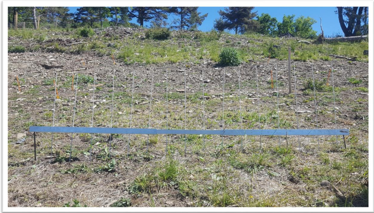
Fig. S3.1. Picture of erosion measurement device
