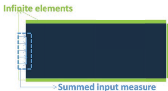
Figure 2.13: Sketch corresponding to solid with infinite elements applied to the boundaries
