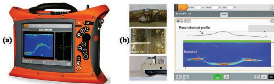
Figure 4.23: (a) Gekko measurement system (b) User interface of Gekko to image using TFM (Credits: M2M)
