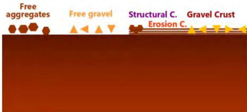
Figure 2.4: Free aggregates and coarse elements, structural crust (embedded aggregates), erosion crust and gravel crust (embedded coarse fragments) (source: (Valentin, 2018))
