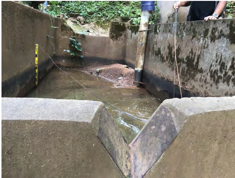
Figure 6.2: A storage attached with combined V-notch and rectangular weir for sediment, bed load, and discharge measurement
