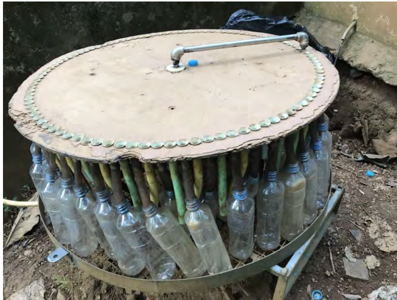
Figure 6.3: Automatic sampler with 600-ml plastic bottles
