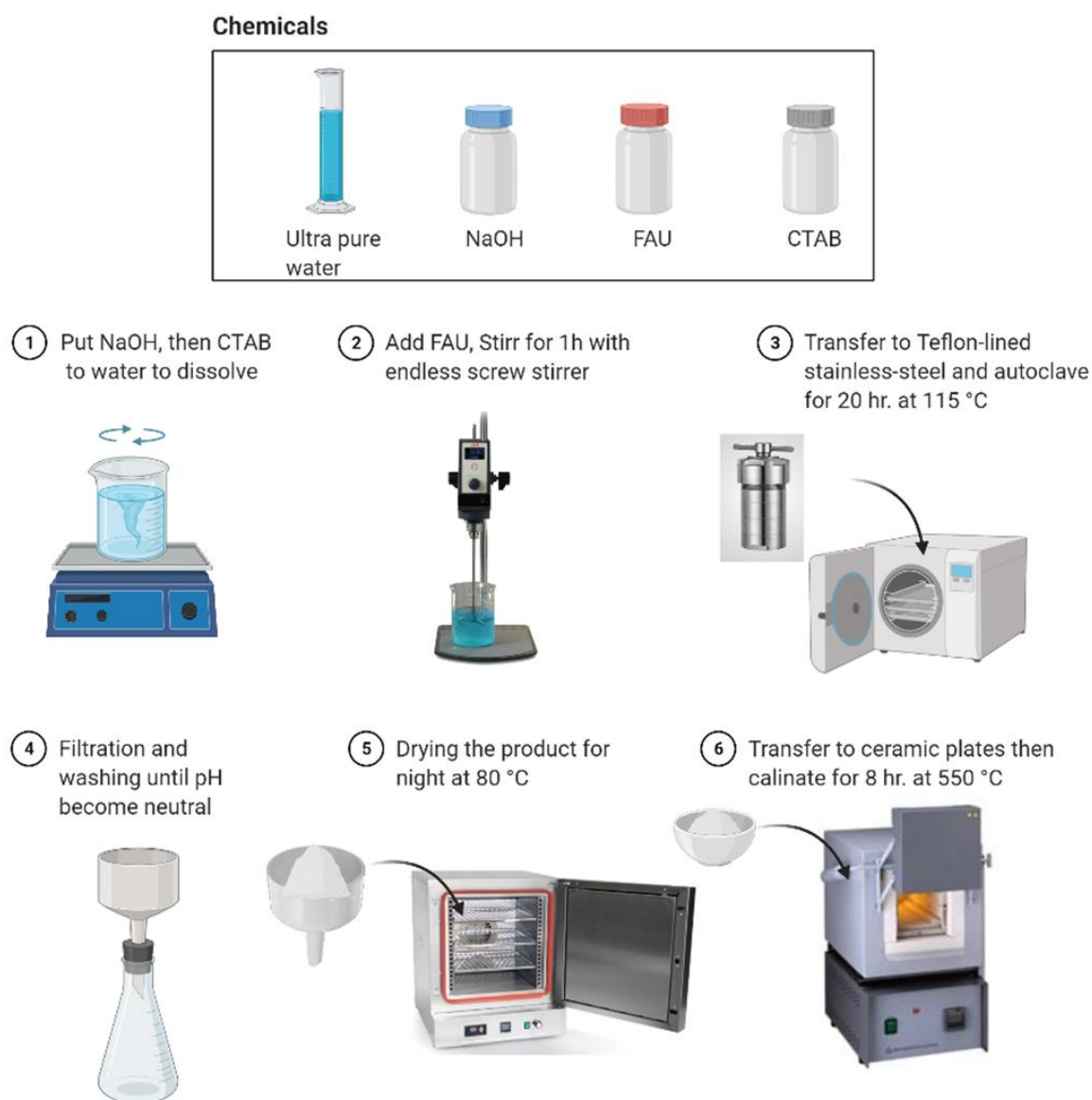
Figure 20 : Procedure used for the modification of FAU material via mixed route (desilication process by NaOH in the presence of structuring agent CTAB).
