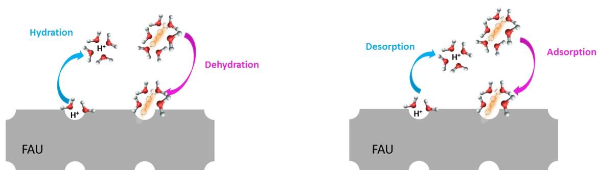
Figure 31 : Major phenomena of the global enthalpy due to adsorption, desorption and displacement (hydration – dehydration).
