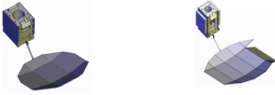
FIGURE 1.15: 6m configuration for deployable RA (left) and 10 m configuration for deployable RA (right).
