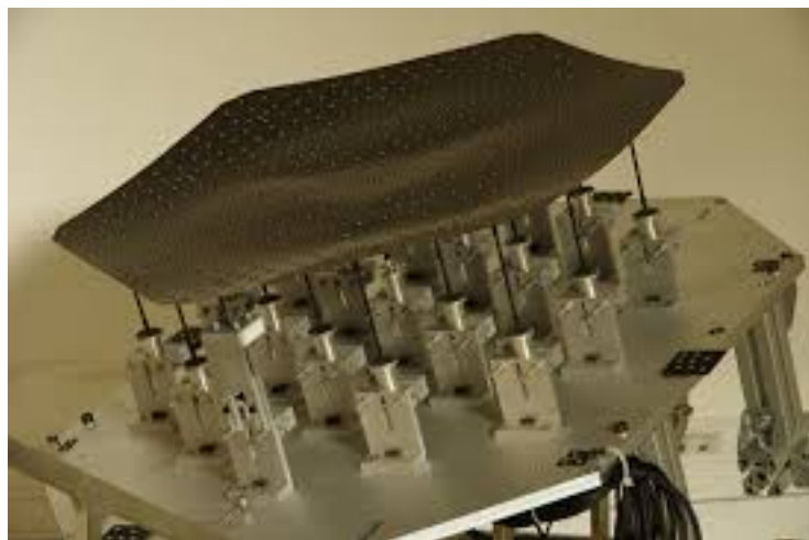
FIGURE 1.22: Reflector antenna with reconfiguration capabilities thanks to actuators.
