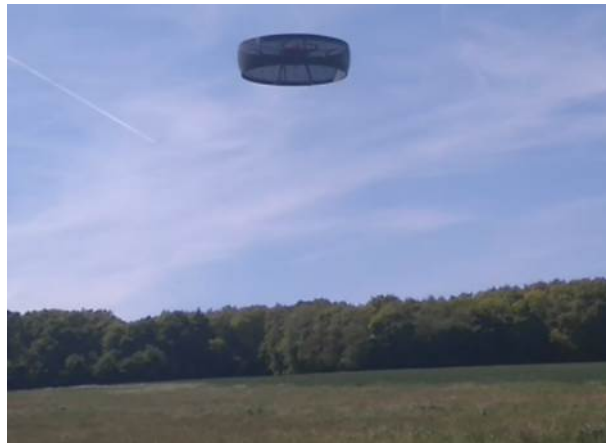
Figure 2.14 – Calibri drone : a specific drone carrying a crown for RCS calibration.
