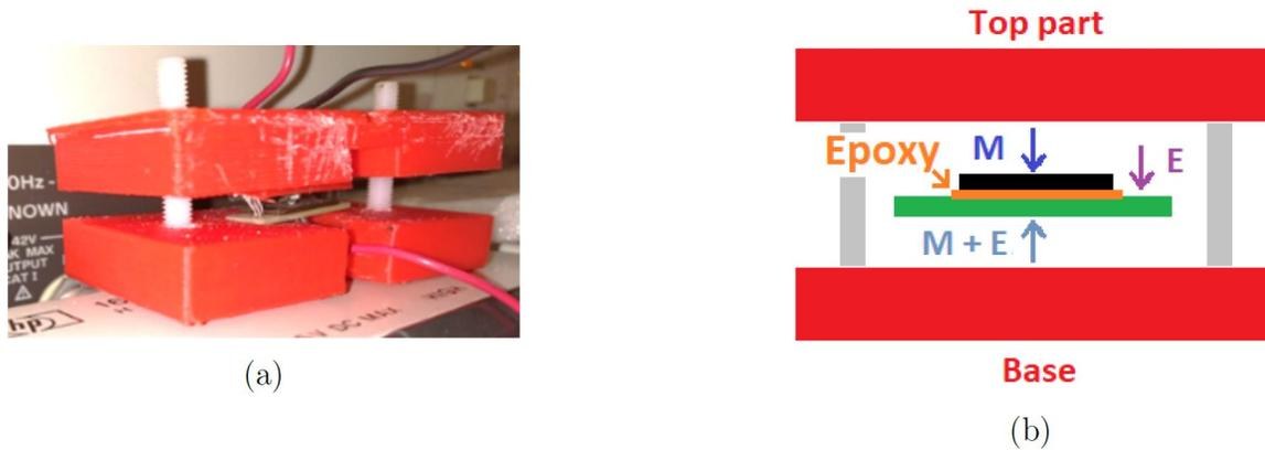
Figure II-5: The sample holder ((a): picture, (b): schematic) "M" denotes a mechanical contact and "E" an electrical contact. "PE" plate in green and "MS" plate in black
